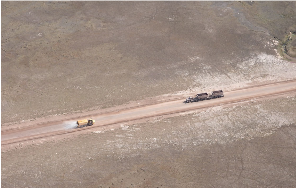
Photo 53. Water Buffalo Applying Dust Suppressant at KM 58 - July
