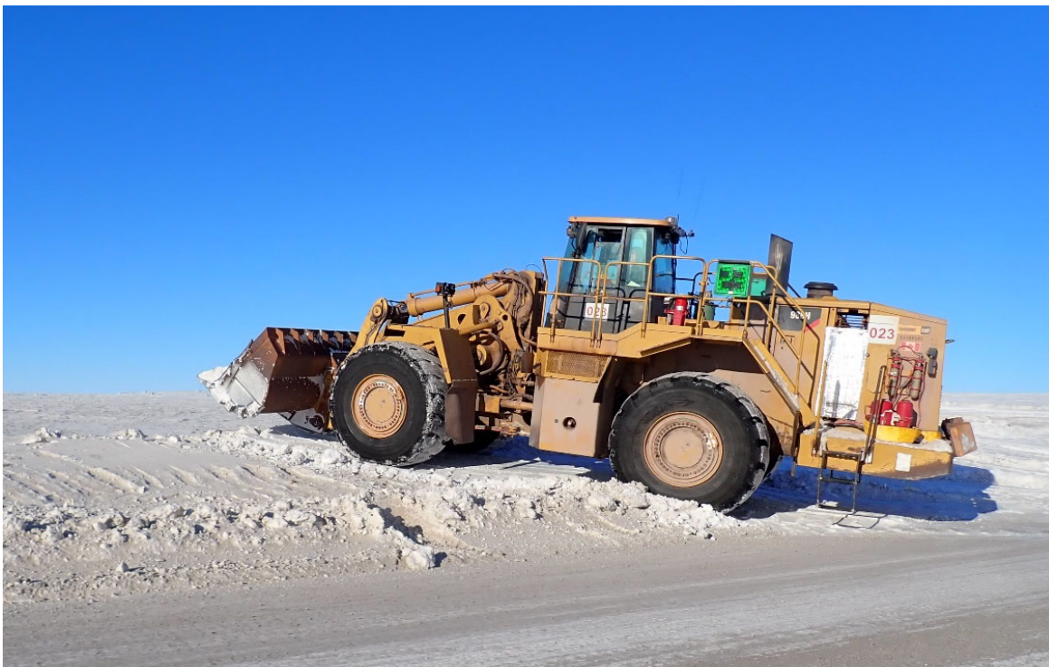
Photo 54. Loader Feathering Snowbank at KM 72 - March
