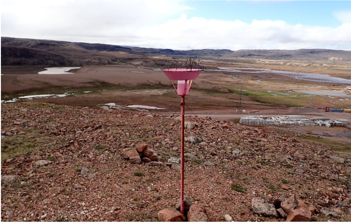
Photo 17. Dustfall Monitoring Station (DF-P-04) – July
