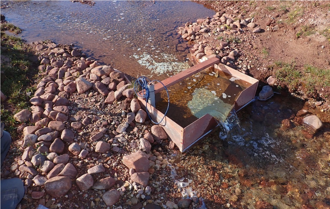
Photo 25. Hydrometric Logger at SNP Site (MP-C-K) – July
