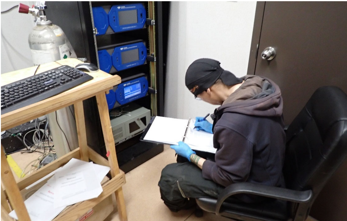
Photo 19. Teledyne T200 NOx Analyzer Unit Inside the Port Site Complex – October
