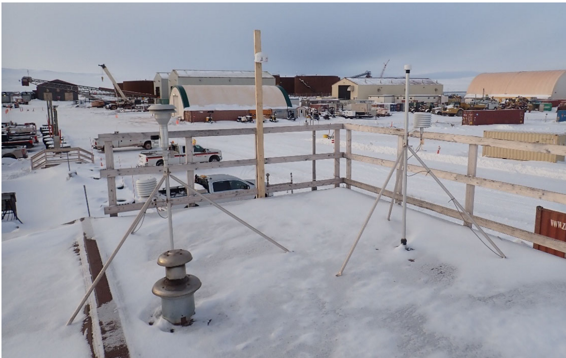
Photo 20. PM 2.5 and TSP Beta Attenuation Monitor Heads on the Port Site Complex – October
