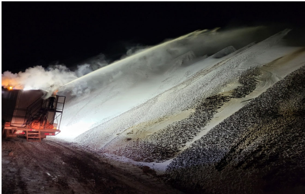
Photo 22. Dust Suppression Application to the Ore Stockpile Pad – January
