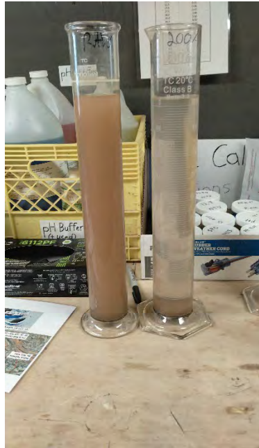
Photo 5. Jar Test Pre-Dosing at the KM 105 Chemical Injection Plant – May 31, 2025
