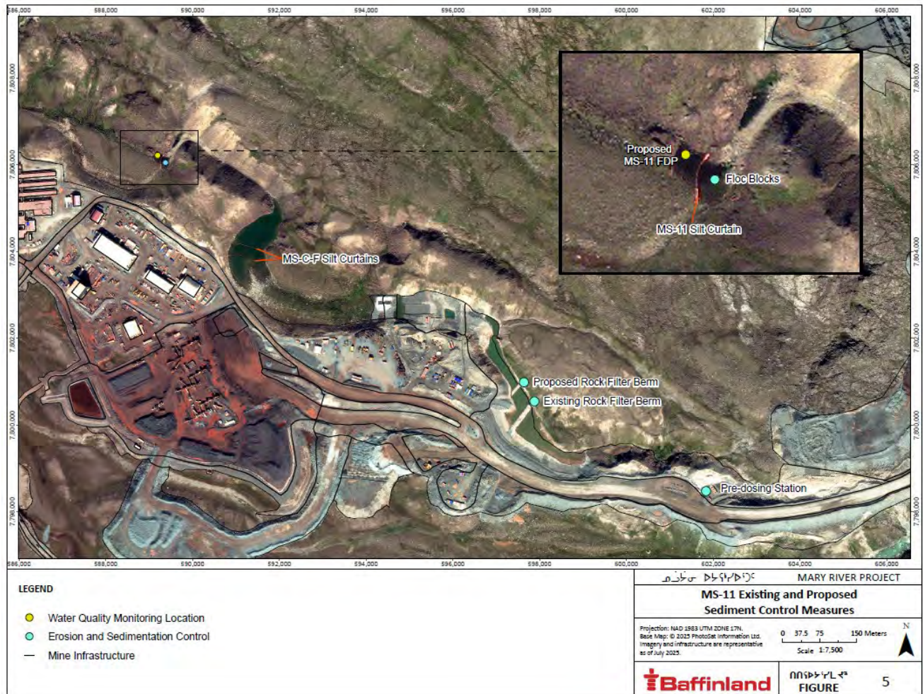
Figure 5 – Sediment Control Measures
