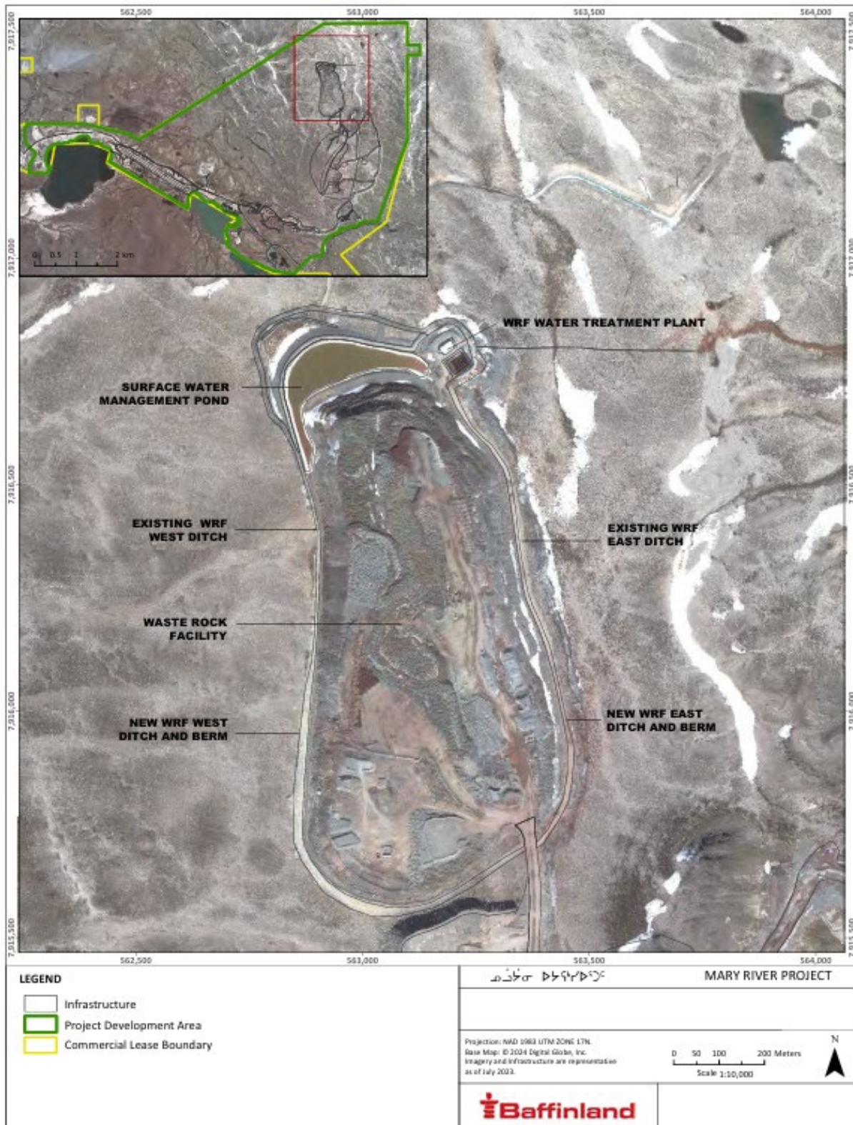
FIGURE 5.2 CURRENT WASTE ROCK FACILITY
