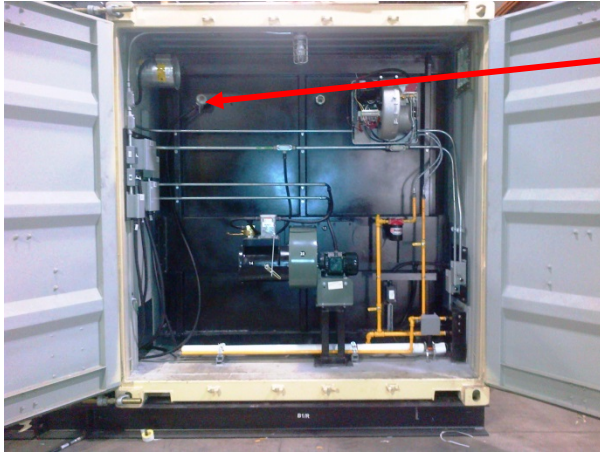
1. Primary Thermocouple (TC1)
