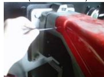
Secondary Burner has 4 screws (2 on each side)
