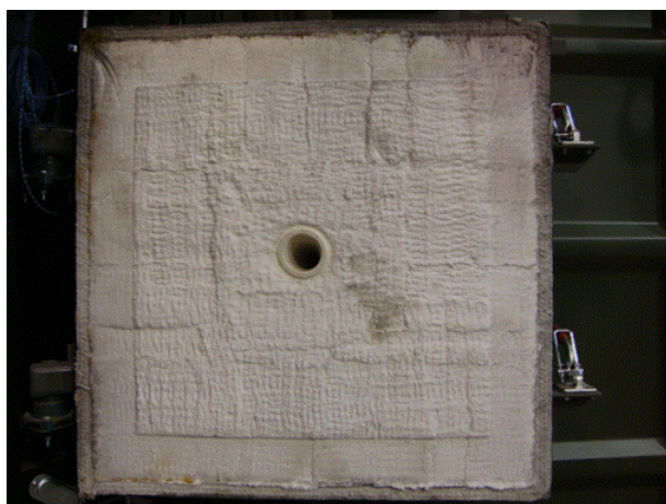
Secondary Door (refractory lined)
