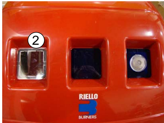
2. Secondary Burner Inspection Window
