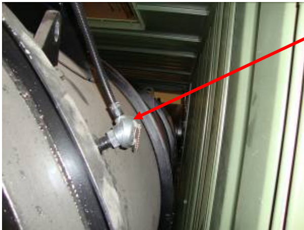
2. Secondary Thermocouple (TC2) on Secondary Chamber Container
