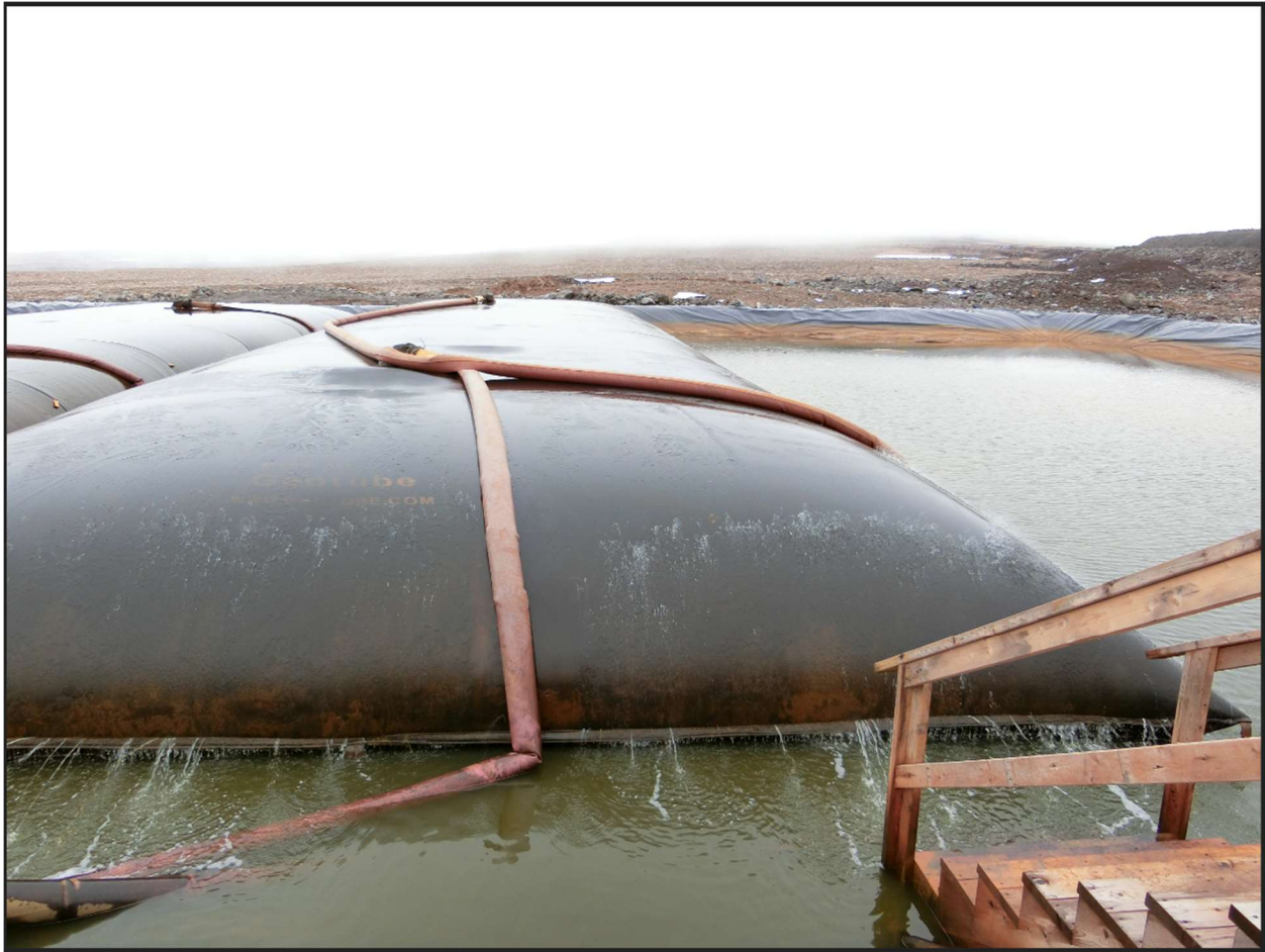
Figure 18 – Geotubes filtering processed water (June 2018)
