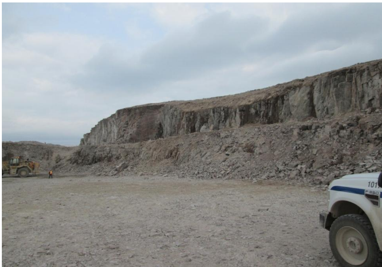
Photo taken looking at the quarry face in the quarry showing the well developed benches and cover removed from atop solid rock.
