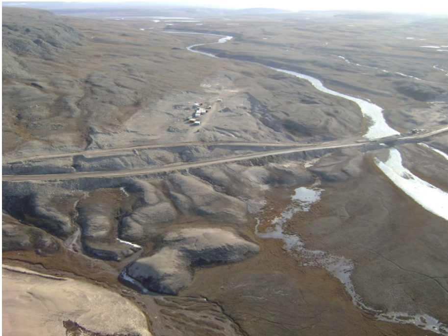
Photo 5A (2593): Pit at KM 61.7 (Figure 8), in 2019, note extensive settlement in southern portion (right side) of the developed pit indicative of the presence of massive ice in portions of this deposit. Note road realignment to improve grade.
