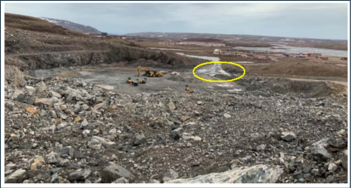
Figure 45: View of QMR2 quarry with area that requires surface water control (yellow circle).
