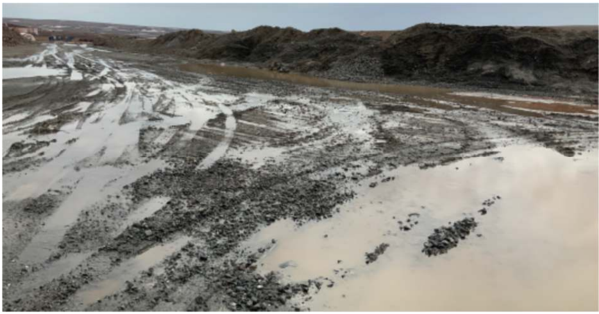
Figure 47: Area that requires improved surface water control at the main level of QMR2 quarry.
