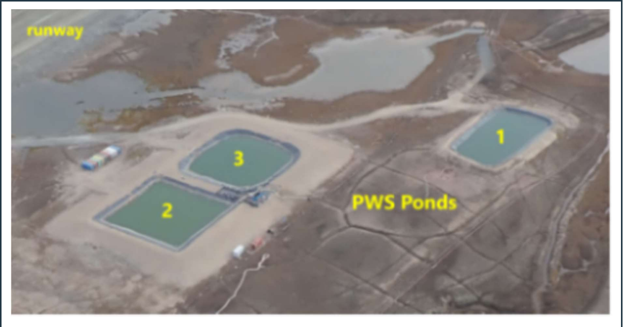
Figure 9: Aerial view of the stable berms around the three PWS ponds. (Historic image to present the layout of the three ponds and to show the robust berms around the facilities).
