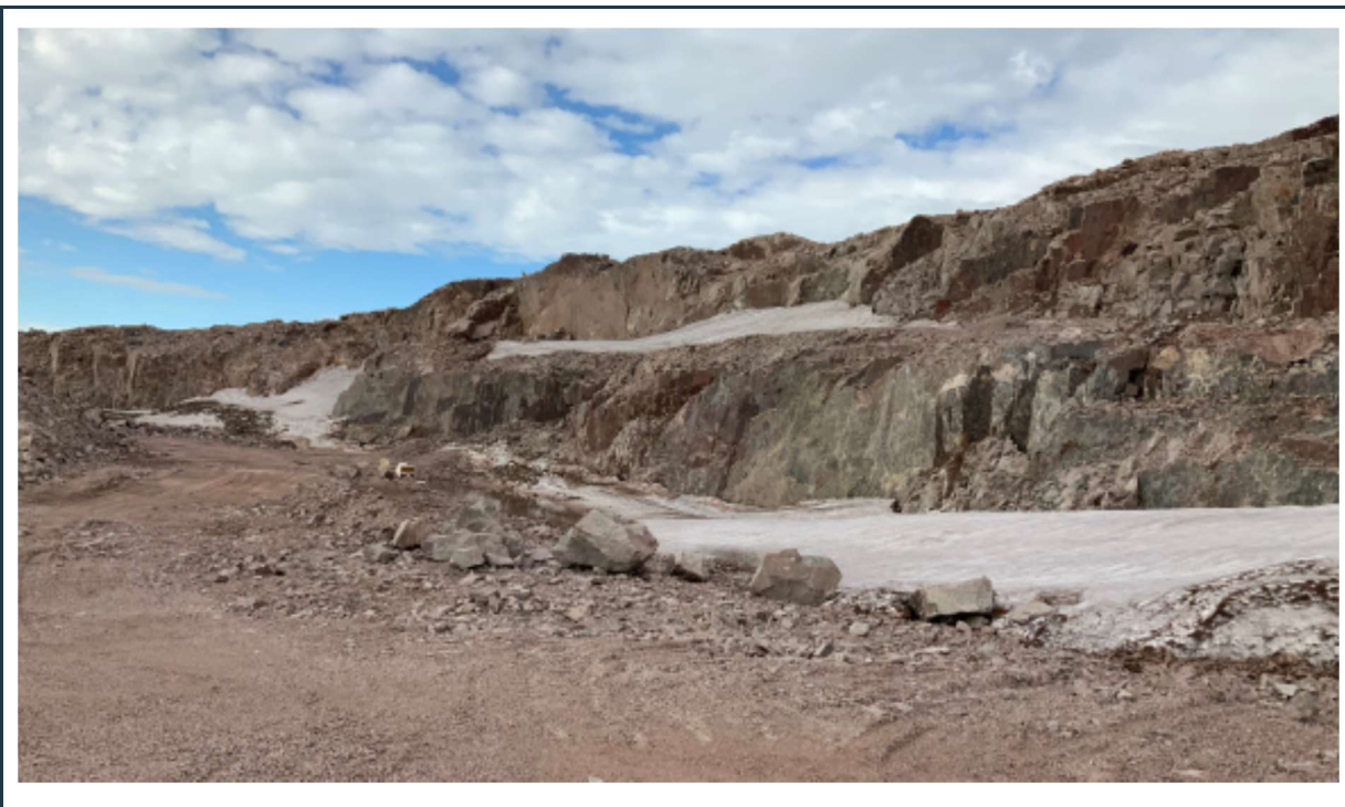
Figure 58: View of stable highwalls with minor weathering and bench erosion in the Q01 rock quarry. Note the accumulated snow on the top of the benches.
