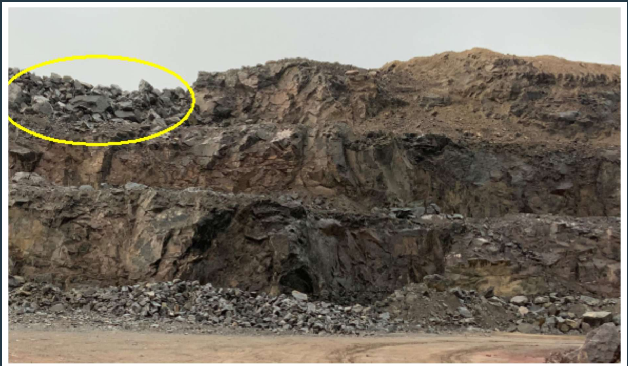
Figure 37: Stable rock face at the upper quarry level, with some potential rolling rock hazard (loose boulders, marked with the yellow circle).
