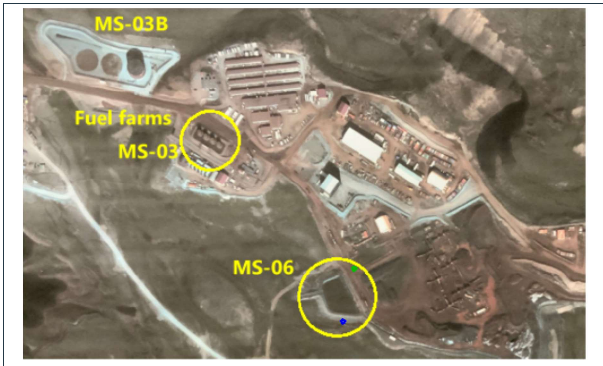
Figure 1: Site layout – Mary River Mine Site - Central Zone with fuel farms and the MS-06 settling pond.
