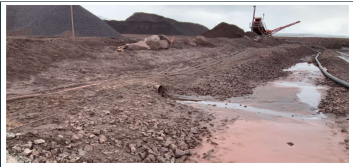
Figure 23: View of the discharge end of the recently cleaned culvert, draining the collected surface water from the crusher area to the MS-06 pond.
