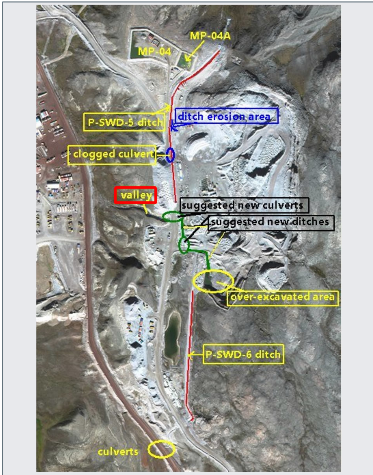
Figure 10: Site layout – Milne Inlet Port Site – South-Eastern Zone. © 2023 Digital Globe, Inc.
