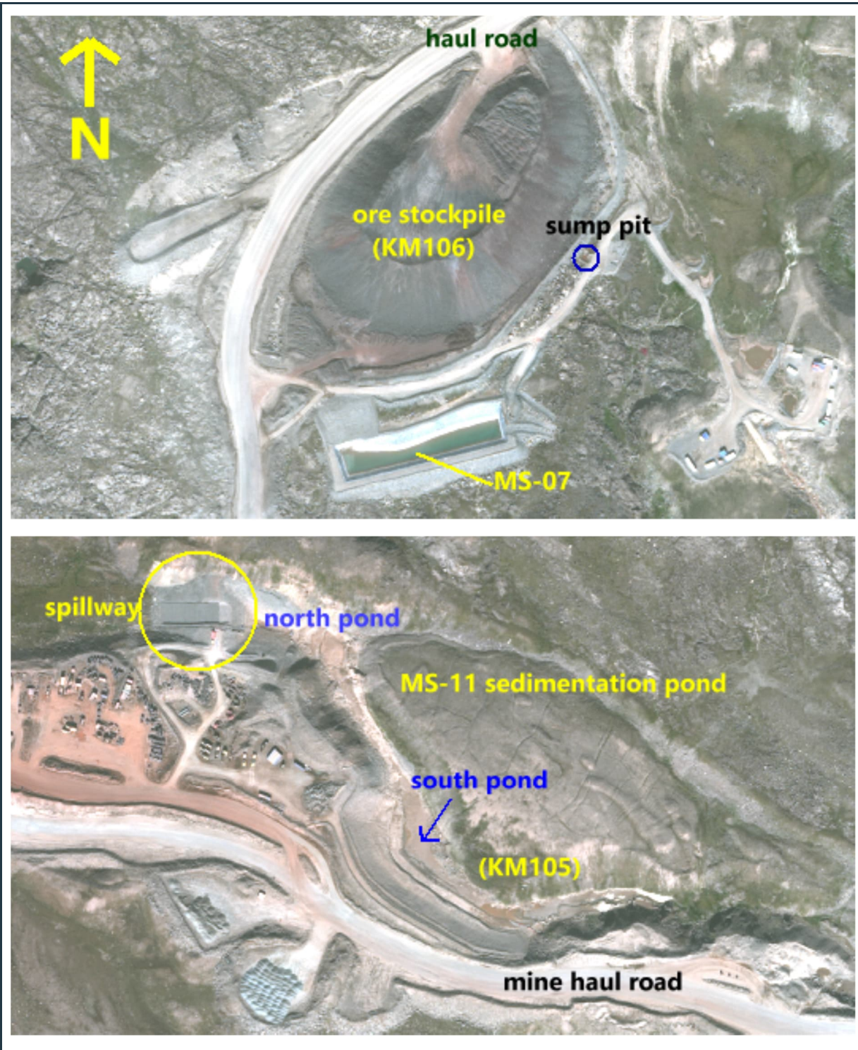
Figure 3: Site layout – Mary River Mine Site – South-Eastern Zone – KM106 run-of-mine ore storage area and KM106/MS-07 and KM105/MS-11 surface water management ponds. © 2023 Digital Globe, Inc.
