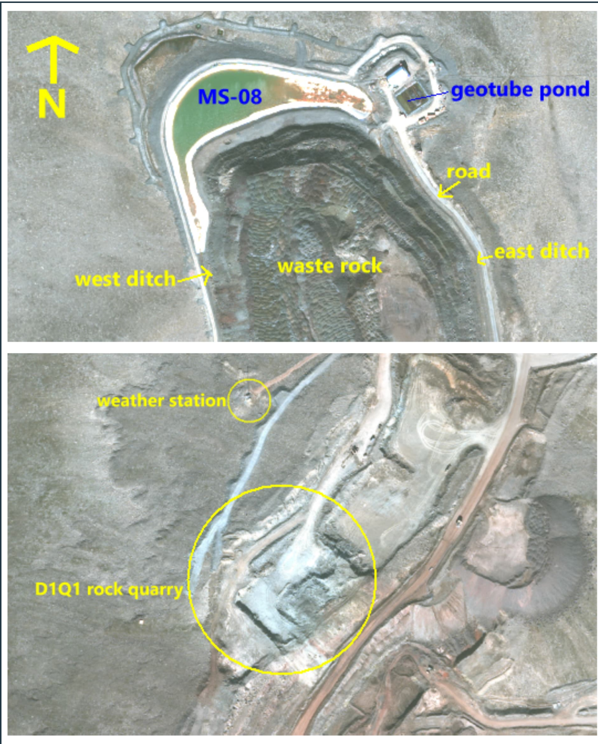
Figure 2: Mary River Site layout – North-Eastern Zone – Waste rock facility with the MS-08 and geotube ponds – D1Q1 rock quarry area. © 2023 Digital Globe, Inc.
