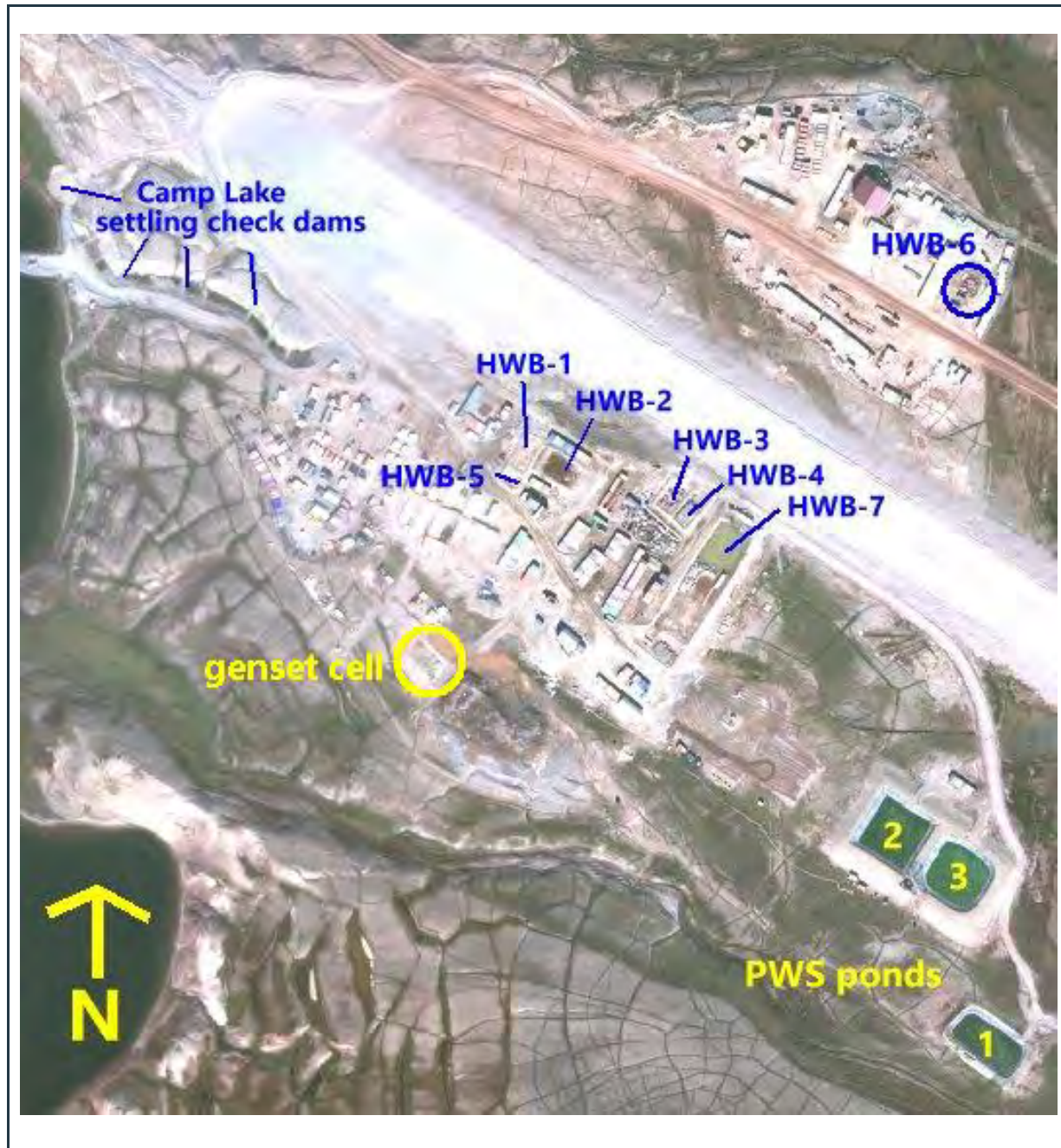
Figure 7: Site layout – Mary River Mine Site - Western Zone – Exploration Camp Polishing Waste Stabilization Ponds (PWSP - MS-MRY04a,b,c), - HWB hazardous waste storage cells (1-7), genset cell, and Camp Lake check dams. © 2023 Digital Globe, Inc.
