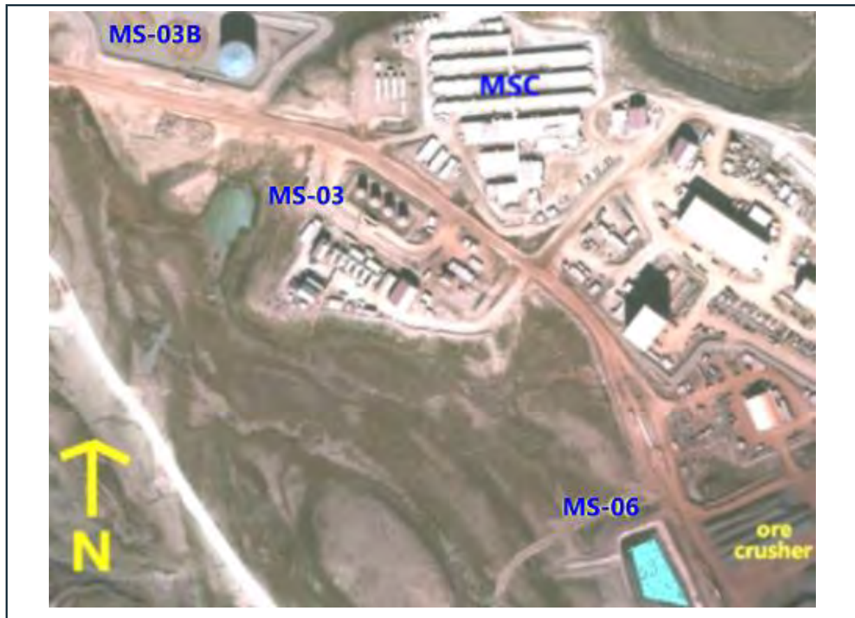
Figure 1: Site layout – Mary River Mine Site - Central Zone – East, showing the MS-03 and MS-03B Bulk Fuel Storage Facility and the MS-06 Ore Stockpile Pond. © 2023 Digital Globe, Inc.
