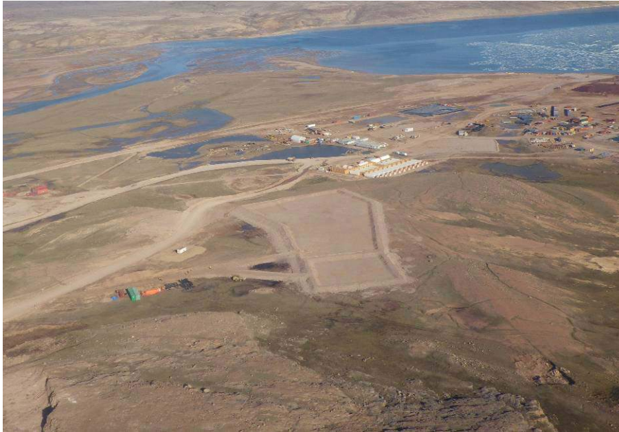
Figure 3: Landfarm package earthworks complete, pre-liner installation [northwest view].
