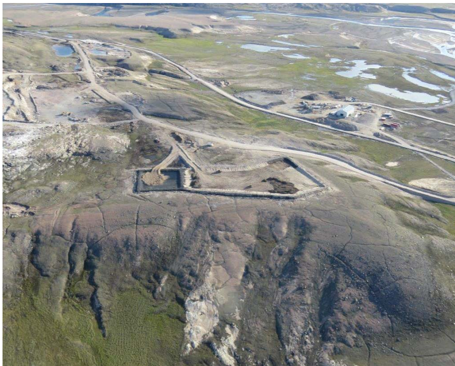
Figure 12: Landfarm Package - Construction Complete [south view].
