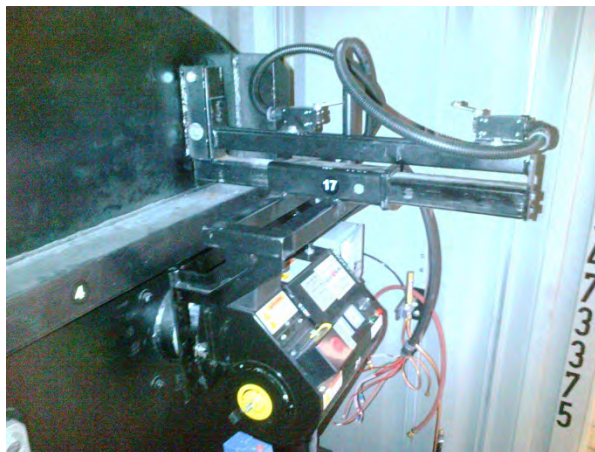
Swing the burner close, secure with pin and push all the way in until front limit switch is made
