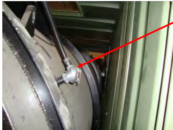
2. Secondary Thermocouple (TC2) on Secondary Chamber Container
