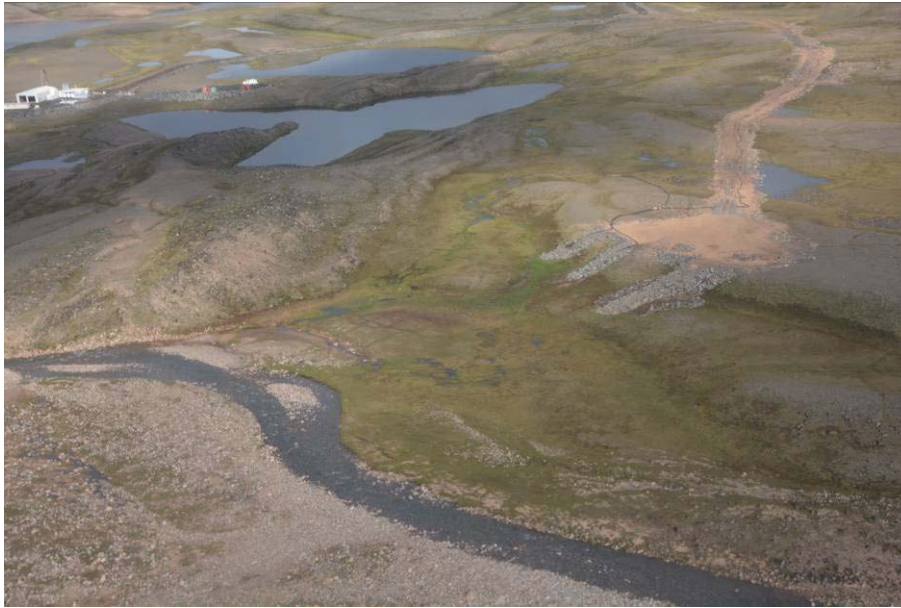
Figure 31: Treated effluent pipeline entering top/right of photo, discharging in three (3) locations: 2 heat traced/ insulated for all-weather use over rip-rap (furthest two rip-rap from camera, left to right), 1 non-insulated for summer discharge only [northwest view]
