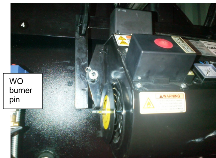
Waste oil burner secured with pin
