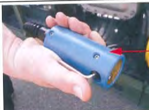
Deadman connector and switch.
