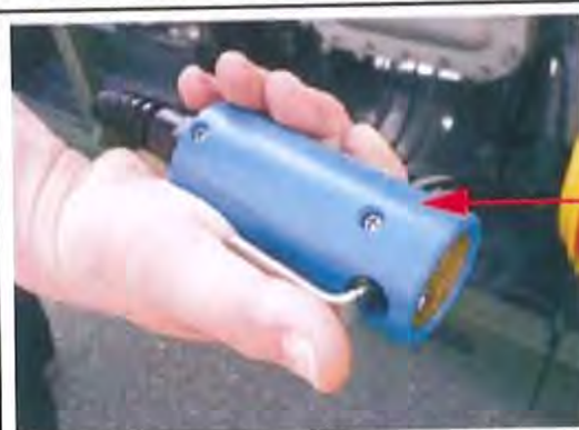
Deadman connector and switch.
