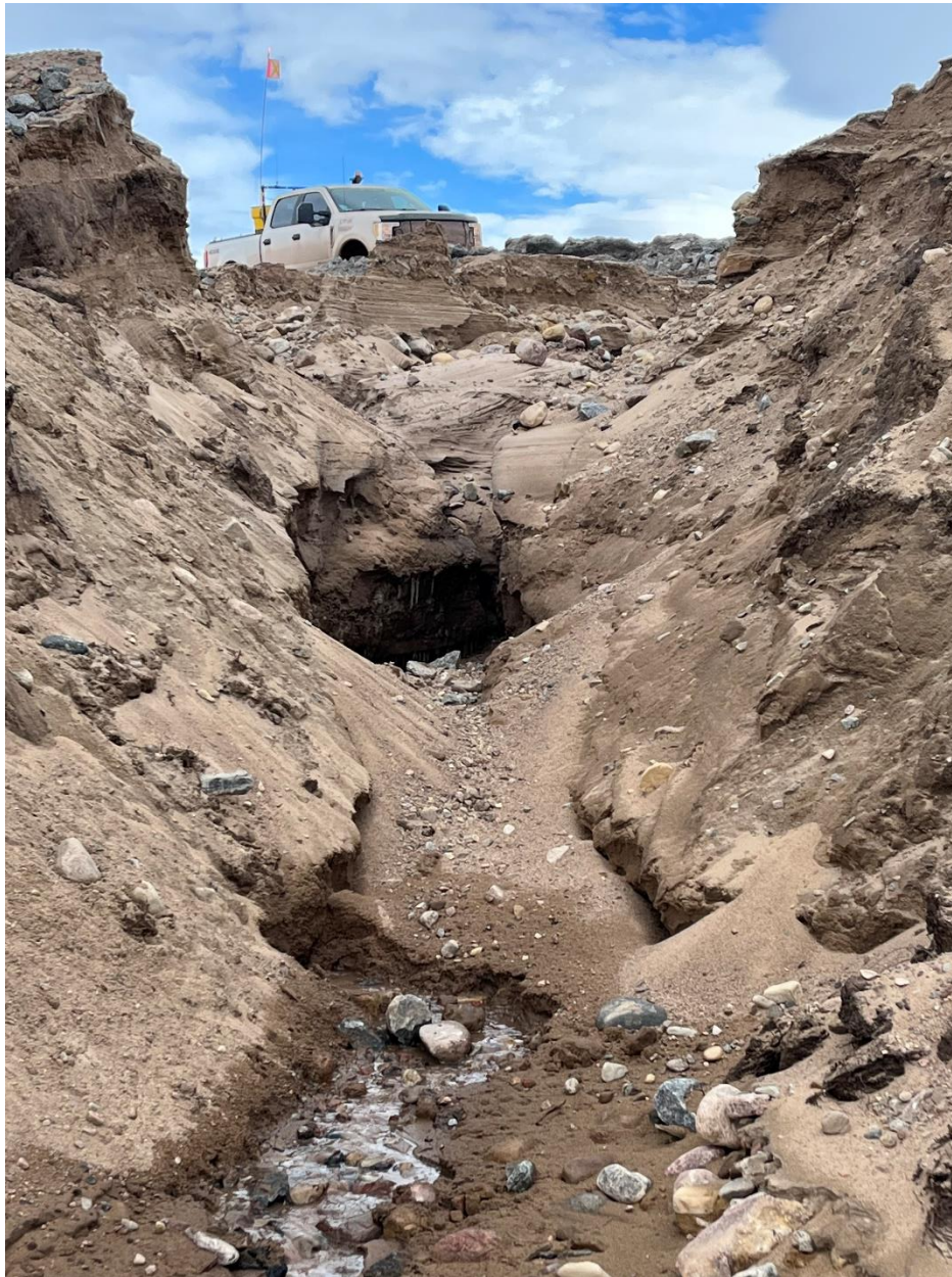
Photo 7 June 16, 2022, erosion cavity; not visible in photo, an ice lens was visible
