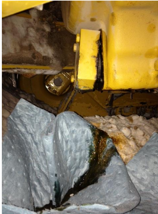
Photo 1: Sheared Inspection Port Cover
