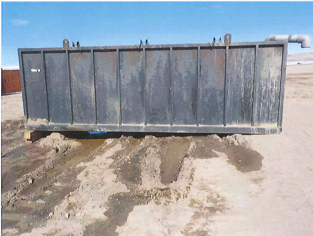
Figure 1: DAF Tank at Location after Release of Oily Water
