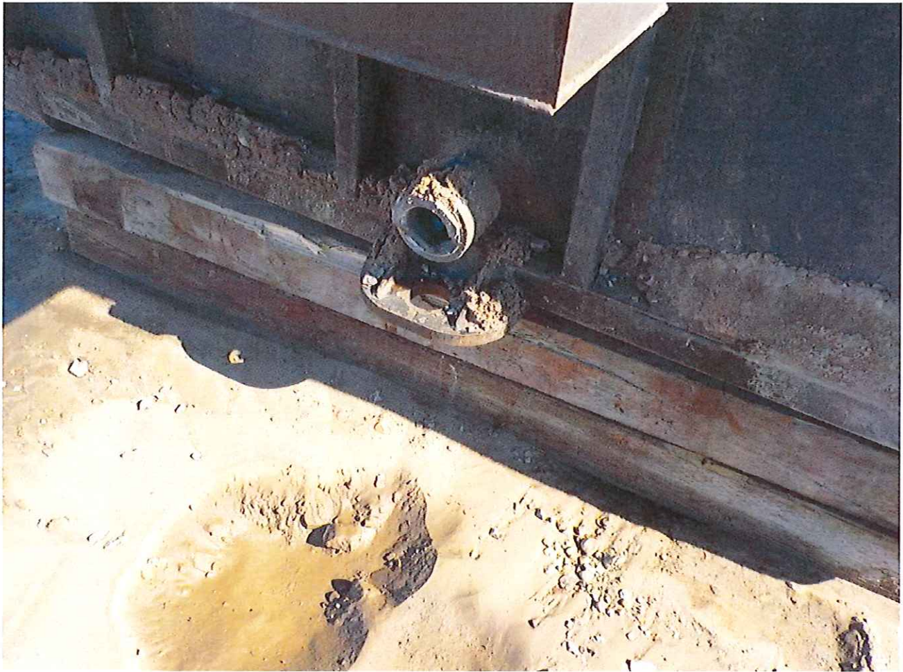
Figure 2: Broken Discharge Pipe (Source of Release of Oily Water)
