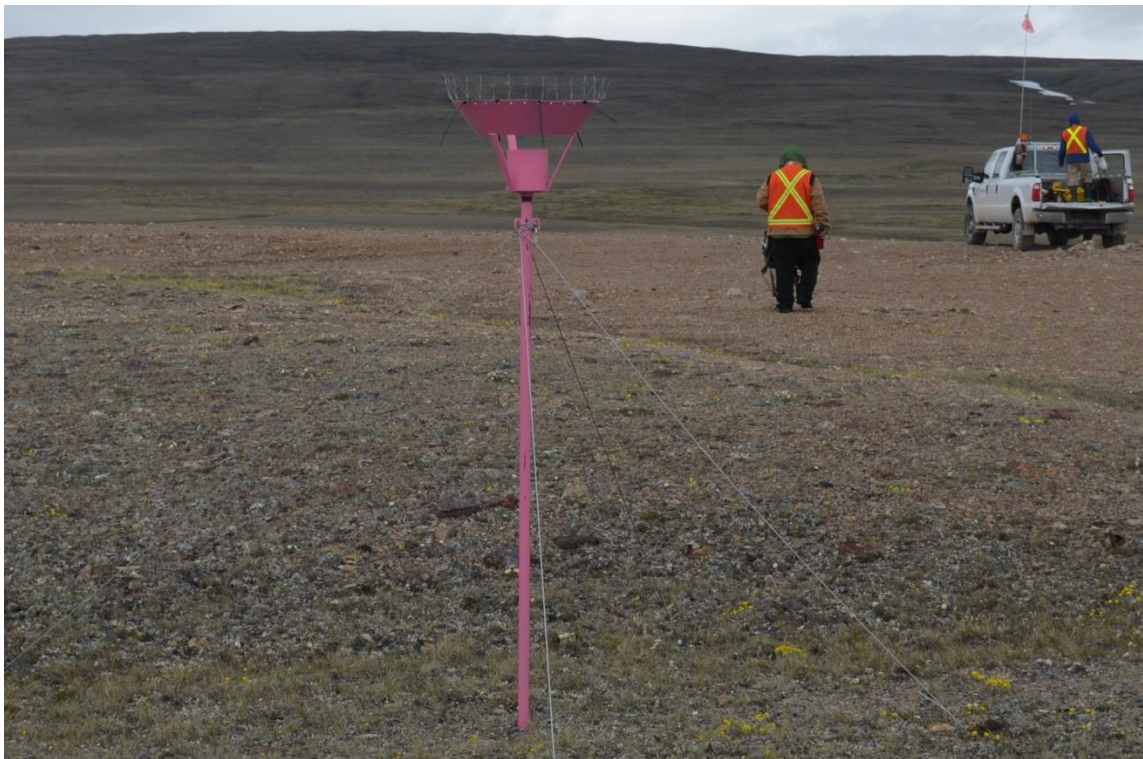
Photo 1. Dust fall collector sampling apparatus, July 10, 2013.
