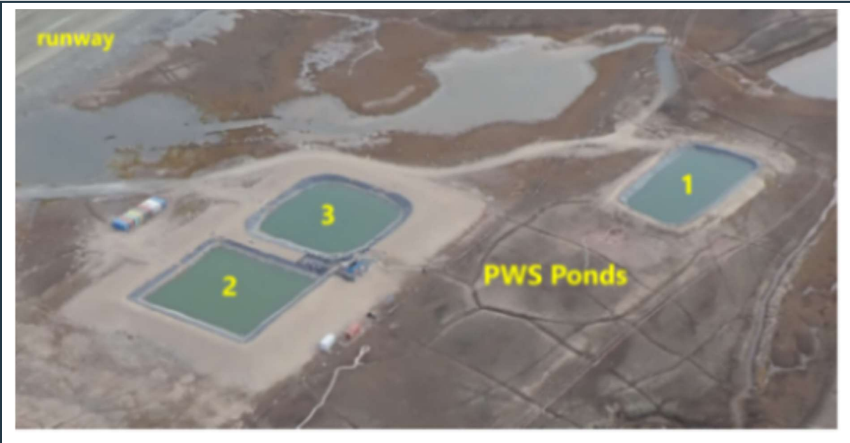
Figure 9: Aerial view of the robust, stable berms around the three PWS ponds. (Historic image to show the layout of the three ponds).
