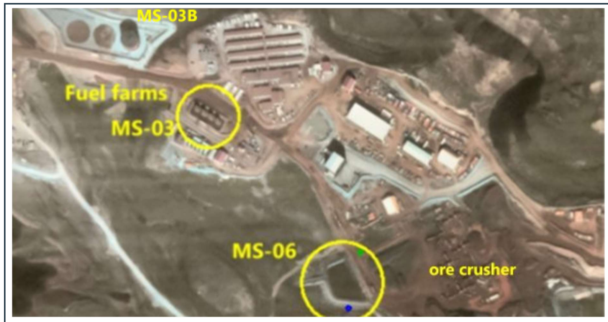
Figure 1: Site layout – Mary River Mine Site - Central Zone with the MS-03 and MS-03B fuel farms and the MS-06 surface water management pond, located near the ore crusher facility.
