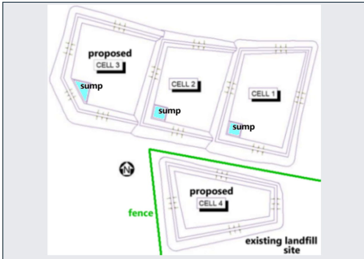
Figure 37: Layout map of the new land-farm cells, adjacent and within the existing landfill facility.
