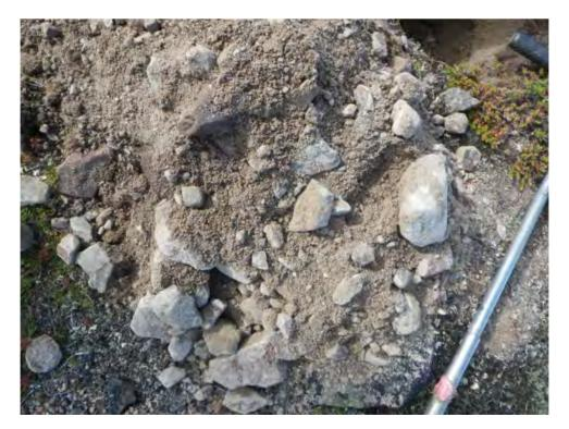
Photo 2: Silty sand till with numerous clasts
