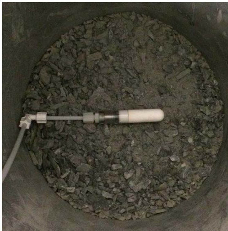
Figure 4: View of the Porous Cup Sampler (Port 1)
