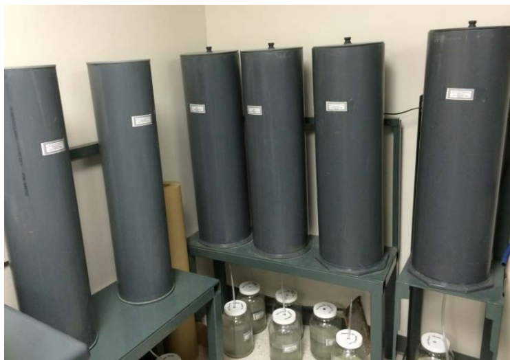
Figure 1: Six Waste Rock Columns Currently Underway.
