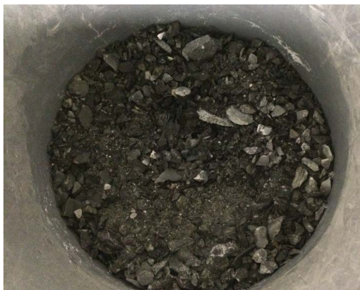
Figure 2: Typical Grain Size (< 9.5 mm) of the Large Column Charge Material
