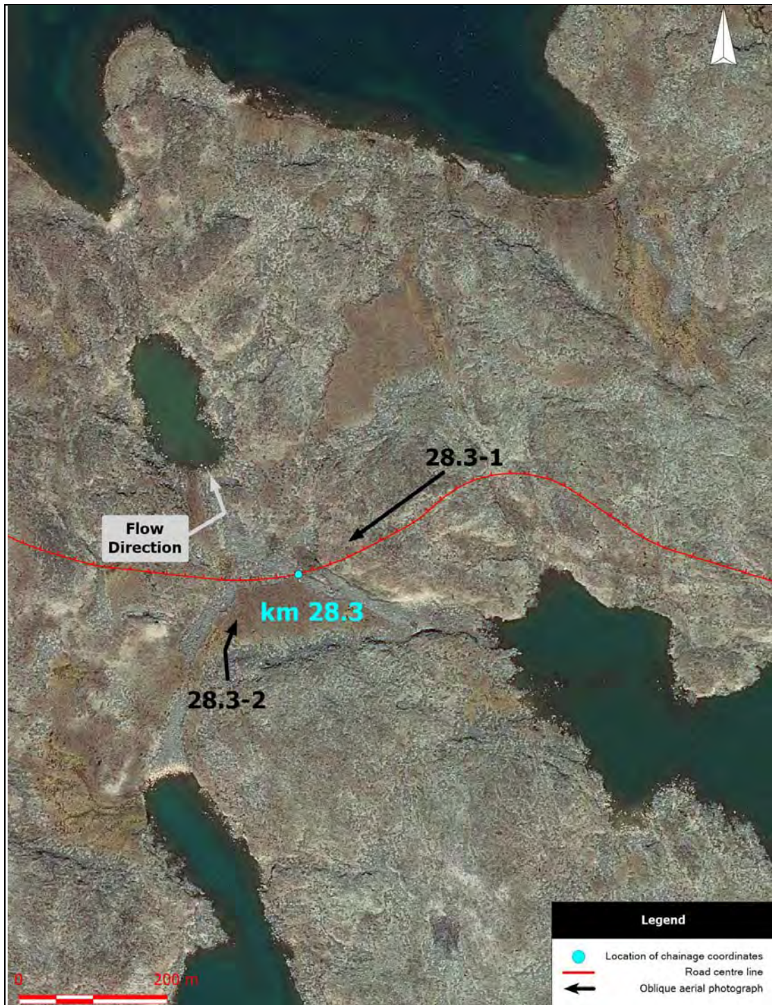
Kilometre 28.3. Aerial photograph showing the road centre line, the location of chainage coordinates provided in Table 3-2, the flow direction, and the location of oblique aerial photographs.
