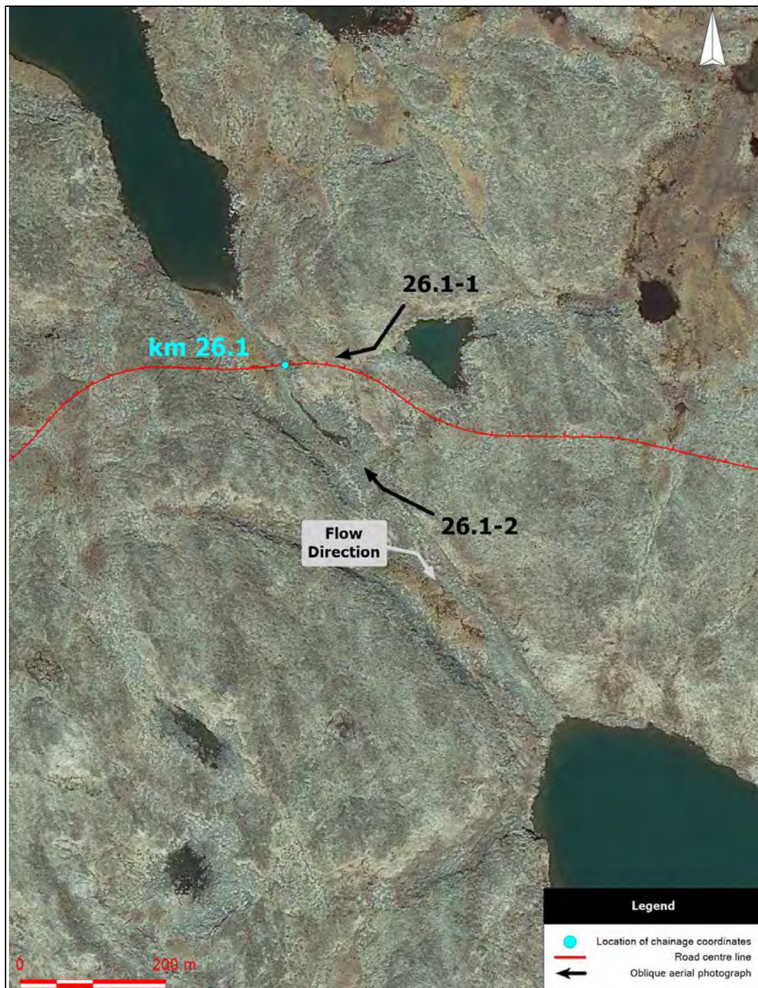
Kilometre 26.1. Aerial photograph showing the road centre line, the location of chainage coordinates provided in Table 3-2, the flow direction, and the location of oblique aerial photographs.
