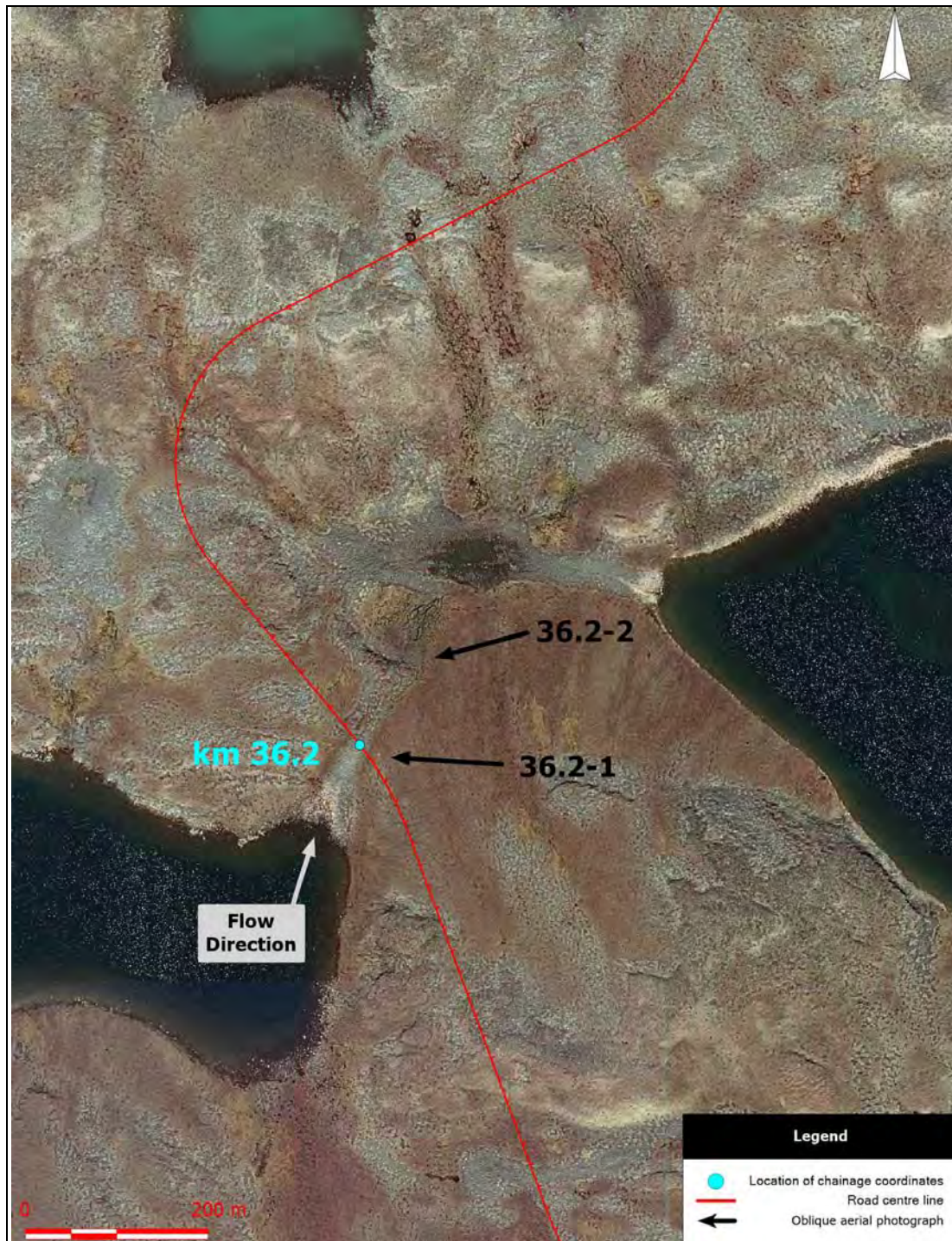
Kilometre 36.2. Aerial photograph showing the road centre line, the location of chainage coordinates provided in Table 3-2, the flow direction, and the location of oblique aerial photographs.
