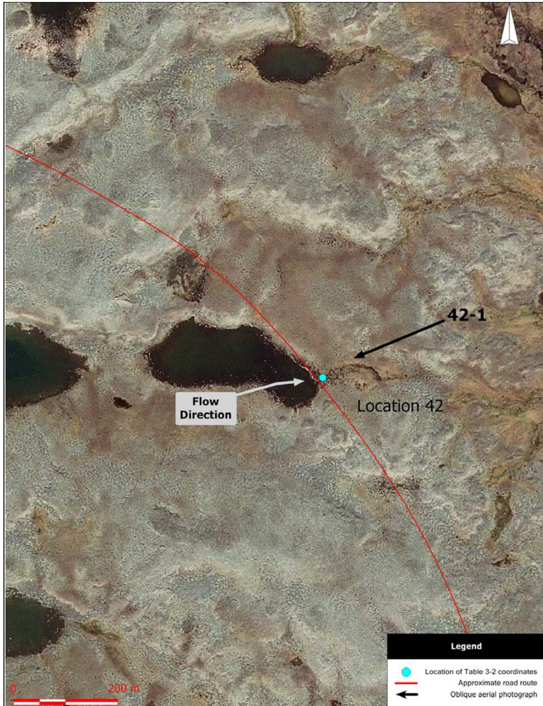
Location 42. Aerial photograph (scale 1:5000) showing the approximate road route, the location of coordinates provided in Table 3-2, the flow direction, and the location of oblique aerial photographs.
