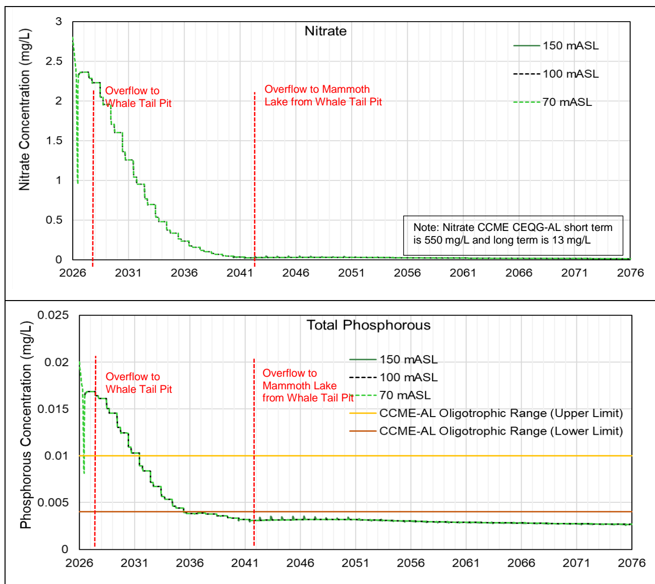
Figure 11: Time-series of nitrate and total phosphorous concentrations at 150 masl, 100 masl and 50 masl in IVR East Basin.
