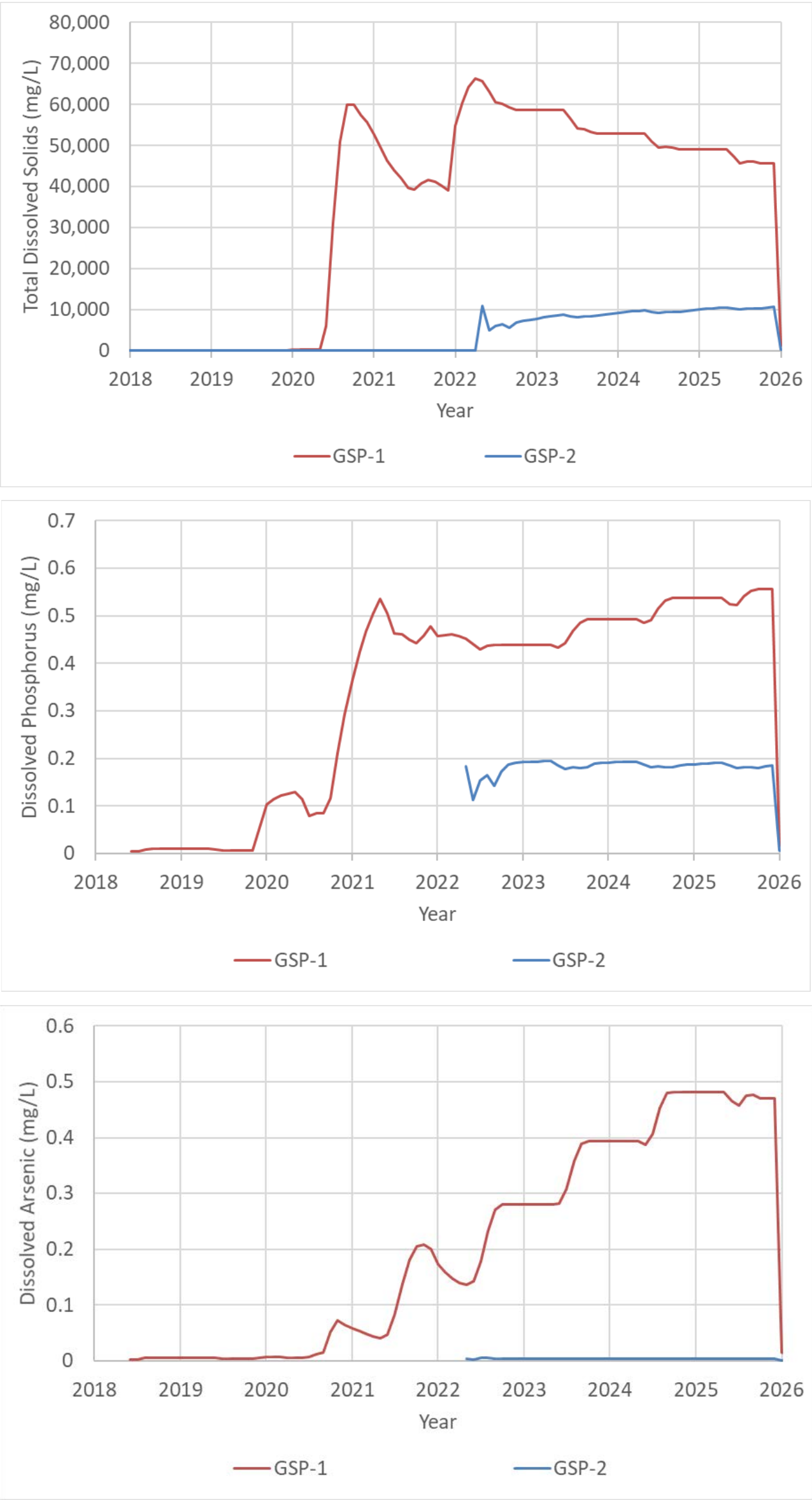
Figure 8: Projected total dissolved solids (TDS) (a), dissolved phosphorus (b) and dissolved arsenic (c) concentrations in the GSP-1 and GSP-2 during operations.
