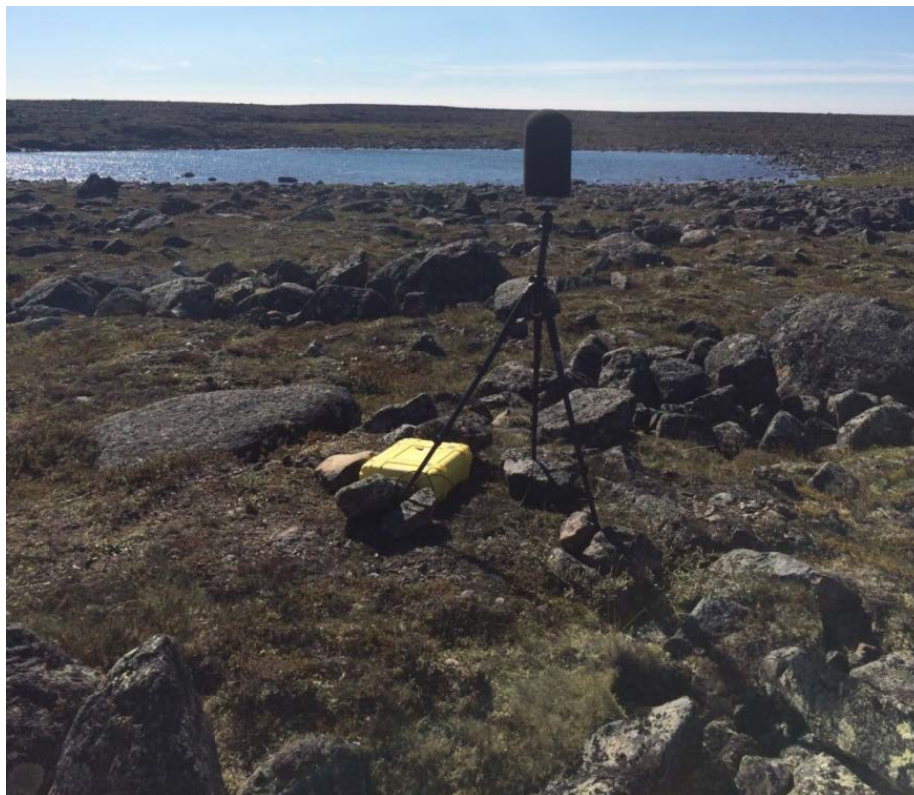
Photo 3-4: Sound Level Meter Deployed at Monitoring Site R9
