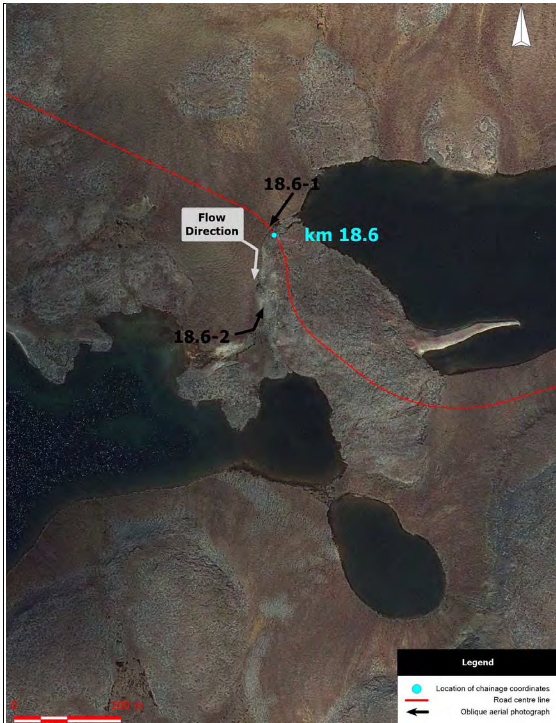
Kilometre 18.6. Aerial photograph showing the road centre line, the location of chainage coordinates provided in Table 3-2, the flow direction, and the location of oblique aerial photographs.
