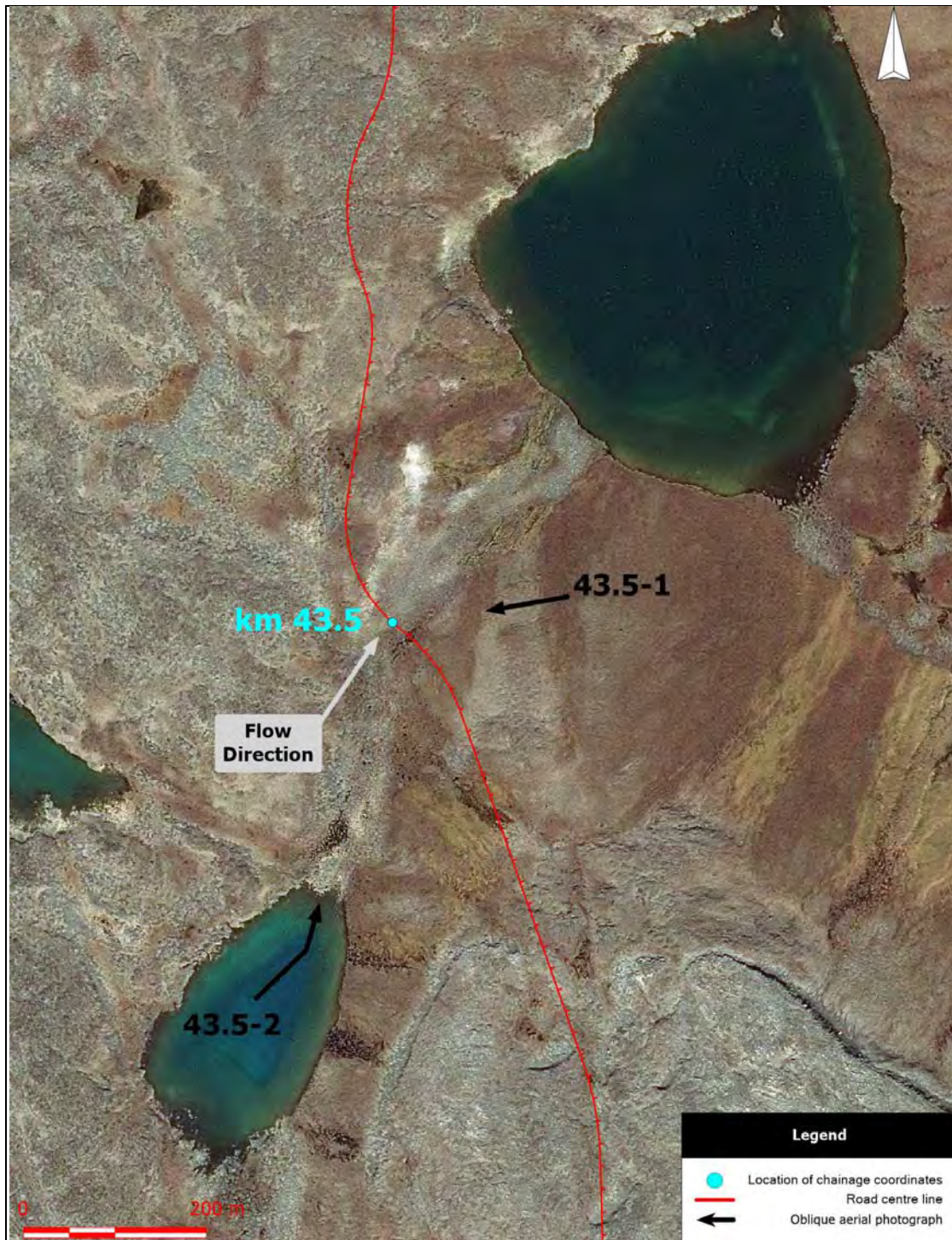
Kilometre 43.5. Aerial photograph showing the road centre line, the location of chainage coordinates provided in Table 3-2, the flow direction, and the location of oblique aerial photographs.
