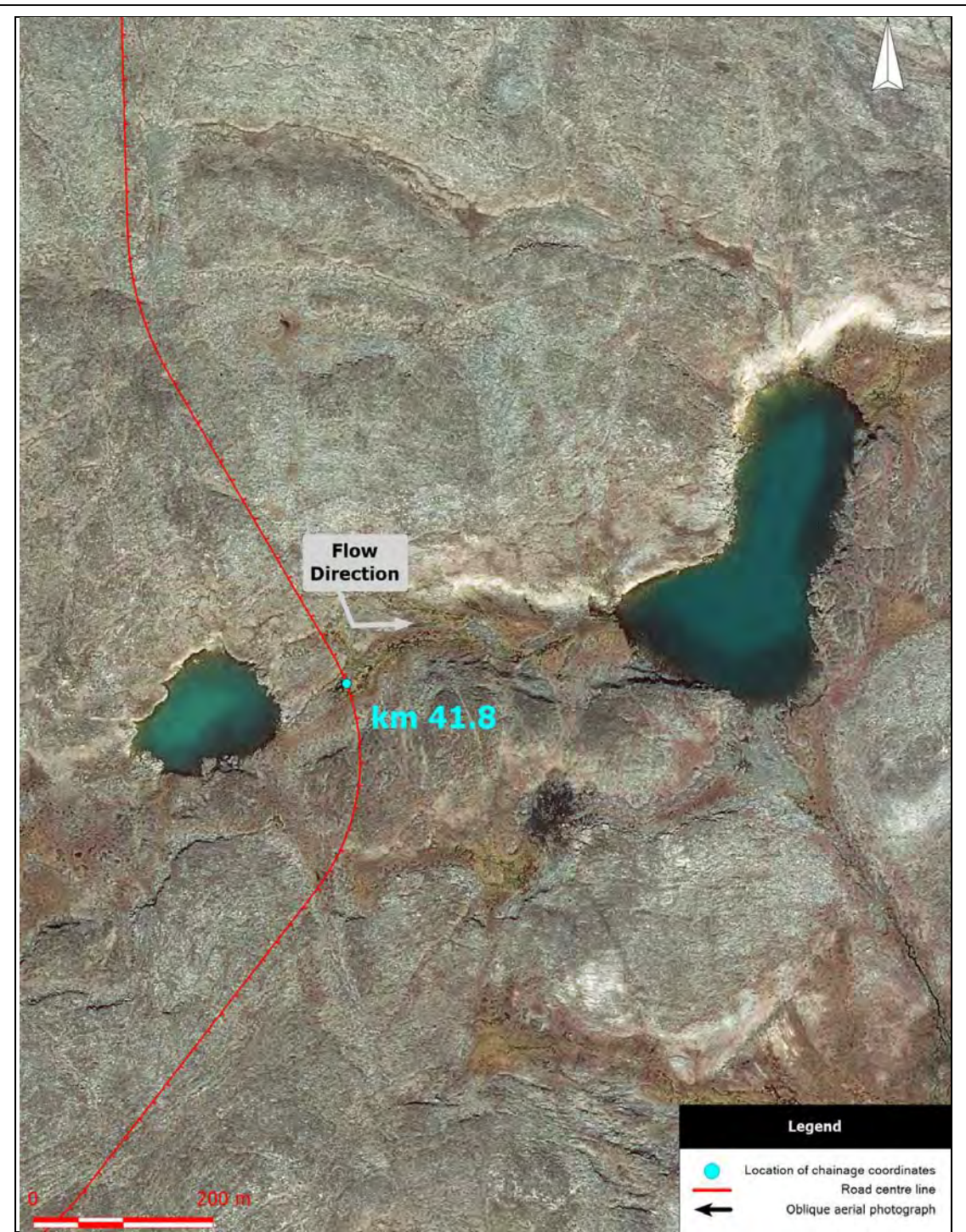
Kilometre 41.8. Aerial photograph showing the road centre line, the location of chainage coordinates provided in Table 3-2, and the flow direction.
