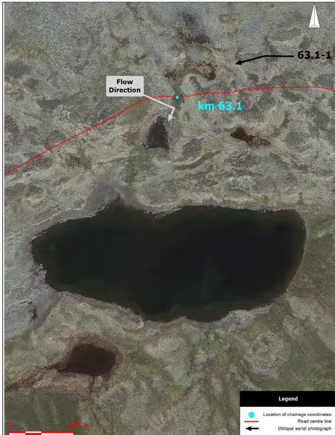
Kilometre 63.1. Aerial photograph showing the road centre line, the location of chainage coordinates provided in Table 3-2, the flow direction, and the location of oblique aerial photographs.
