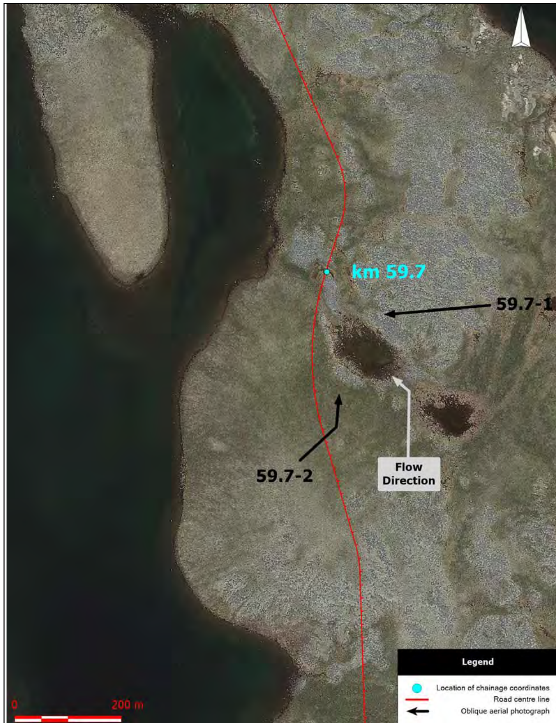
Kilometre 59.7. Aerial photograph showing the road centre line, the location of chainage coordinates provided in Table 3-2, the flow direction, and the location of oblique aerial photographs.
