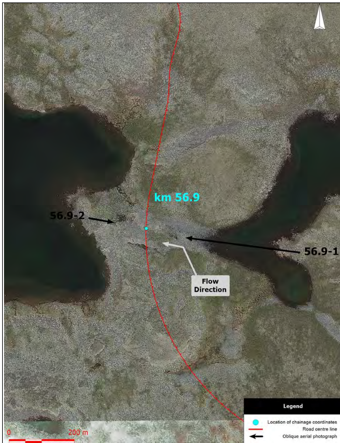
Kilometre 56.9. Aerial photograph showing the road centre line, the location of chainage coordinates provided in Table 3-2, the flow direction, and the location of oblique aerial photographs.
