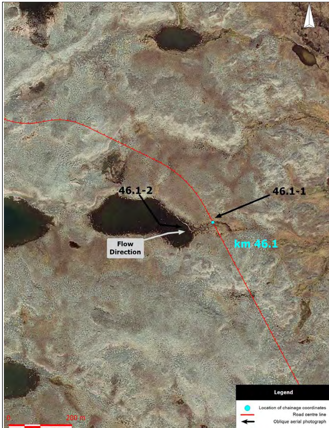
Kilometre 46.1. Aerial photograph showing the road centre line, the location of chainage coordinates provided in Table 3-2, the flow direction, and the location of oblique aerial photographs.
