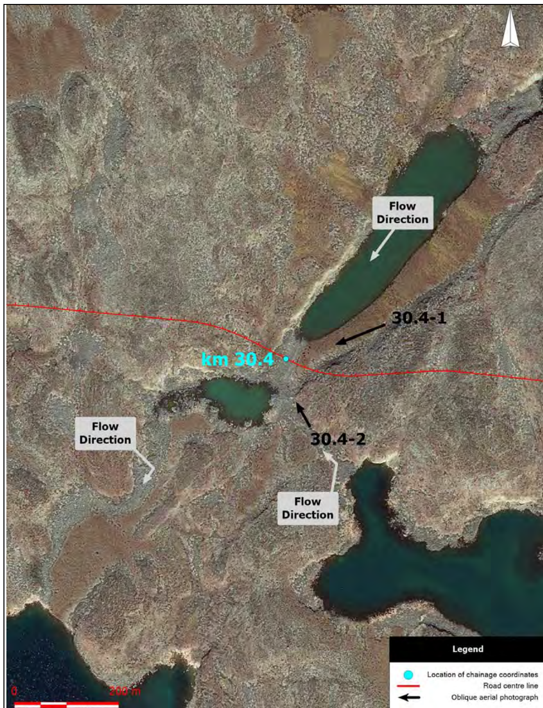
Kilometre 30.4. Aerial photograph showing the road centre line, the location of chainage coordinates provided in Table 3-2, the flow direction, and the location of oblique aerial photographs.
