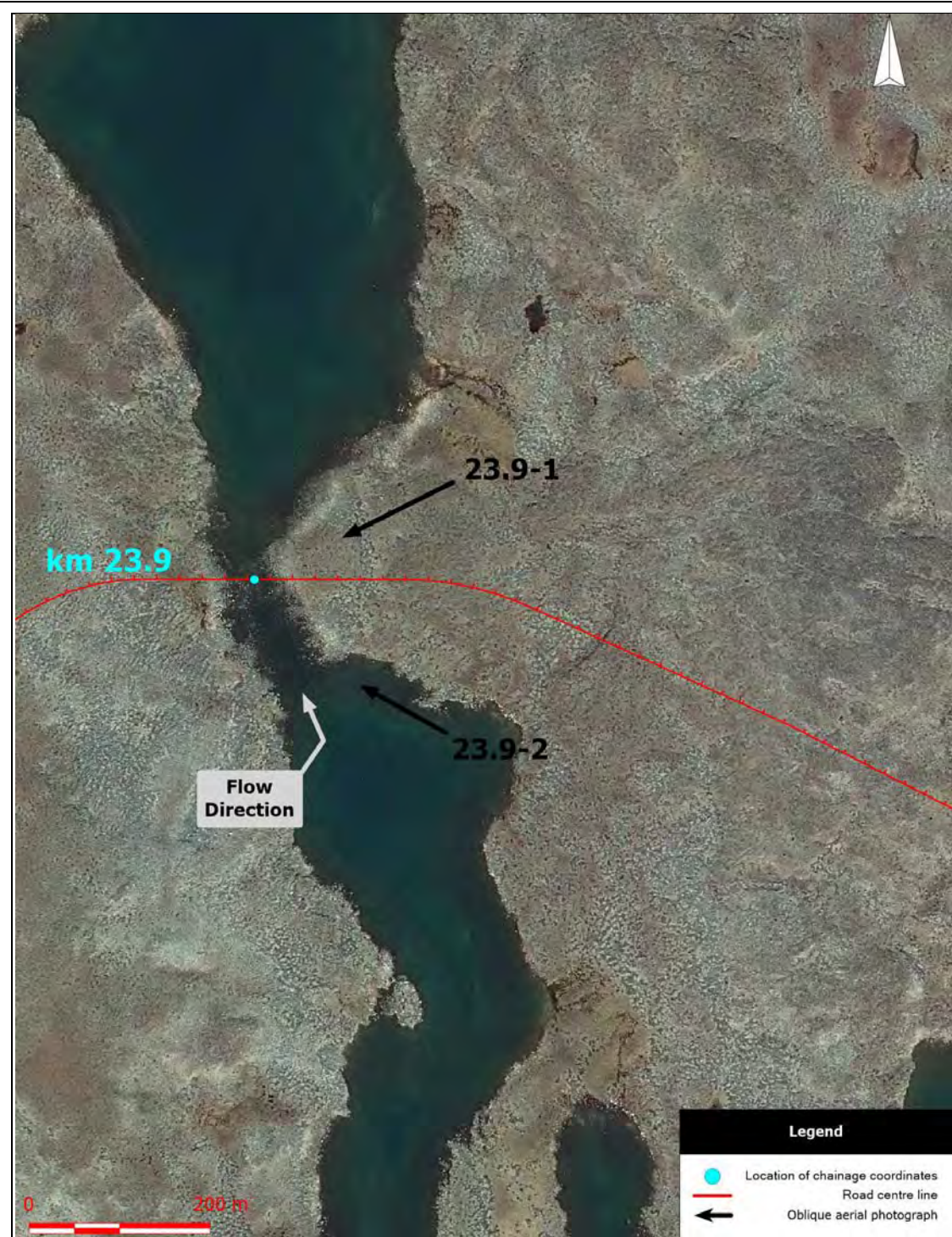
Kilometre 23.9. Aerial photograph showing the road centre line, the location of chainage coordinates provided in Table 3-2, the flow direction, and the location of oblique aerial photographs.
