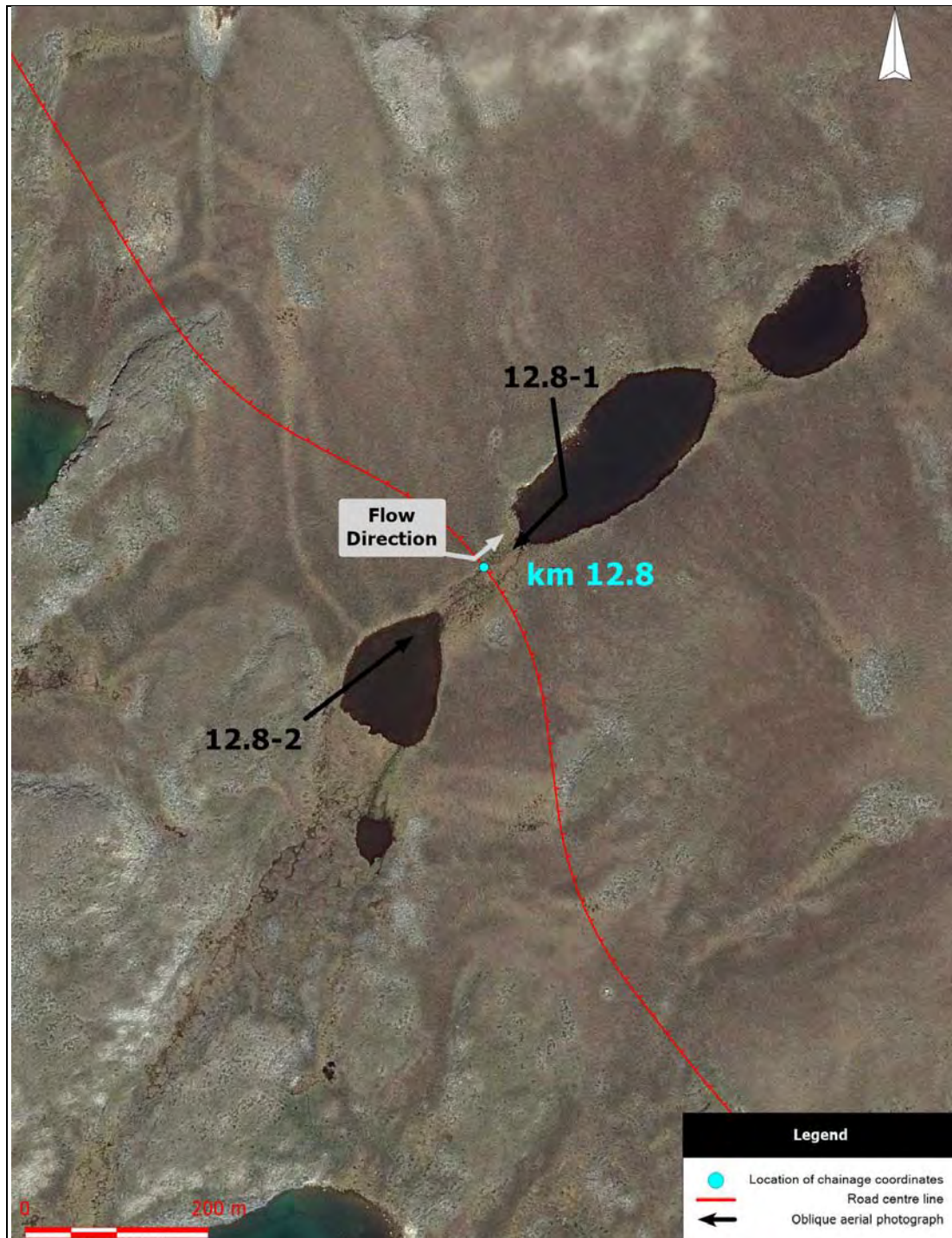
Kilometre 12.8. Aerial photograph showing the road centre line, the location of chainage coordinates provided in Table 3-2, the flow direction, and the location of oblique aerial photographs.
