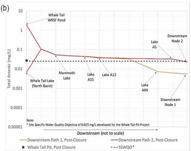
Downstream water quality with 4 m active thaw depth (without treatment) assuming 2% arsenic leaching materials in WRSF cover.
