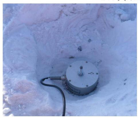
Figure 4: Transducer tightened with a nut
