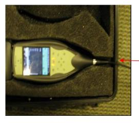
Extend microphone extension cord over notched portion of protective case.
