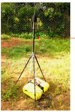
Tape microphone extension cord along tripod.
