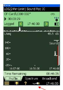
External power symbol indicating that external power is connected.
