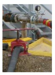
Guillotine was pre-installed as per discharge protocol and it was closed right after the call of the leak
