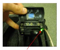
Check 2250 Analyzer LED for power.
