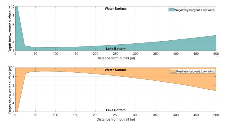
Figure 3.2: Profile View of the Predicted Plumes for Positively and Negatively Buoyant Summer Cases
