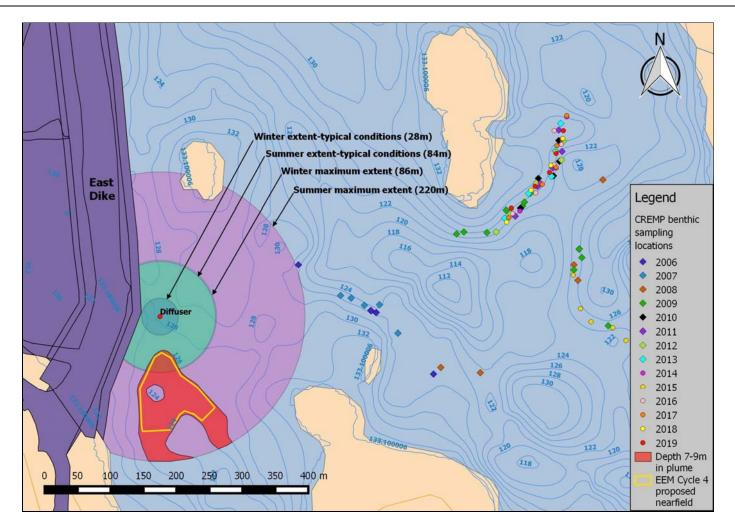
Figure 2-2. Diffuser (discharge point) location and modeled plume extents under typical conditions and worst-case conditions at the maximum measured discharge rate for the period February 18, 2017, through December 31, 2019.
