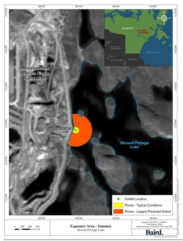
Figure A.1: Summer Conditions - Region of Second Portage Lake where the predicted effluent concentration is greater than 1%. Plume extents shown for typical conditions and for conditions producing the largest plume for flow of 10.8 L/s.
