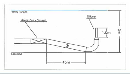
Figure 2.1: Schematic of Diffuser and Discharge Pipe (Agnico, 2014)
