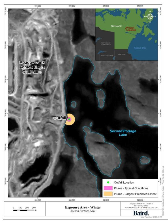
Figure A.2: Winter Conditions - Region of Second Portage Lake where the predicted effluent concentration is greater than 1%. Plume extents shown for typical conditions and for conditions producing the largest plume for flow of 7.9 L/s.
