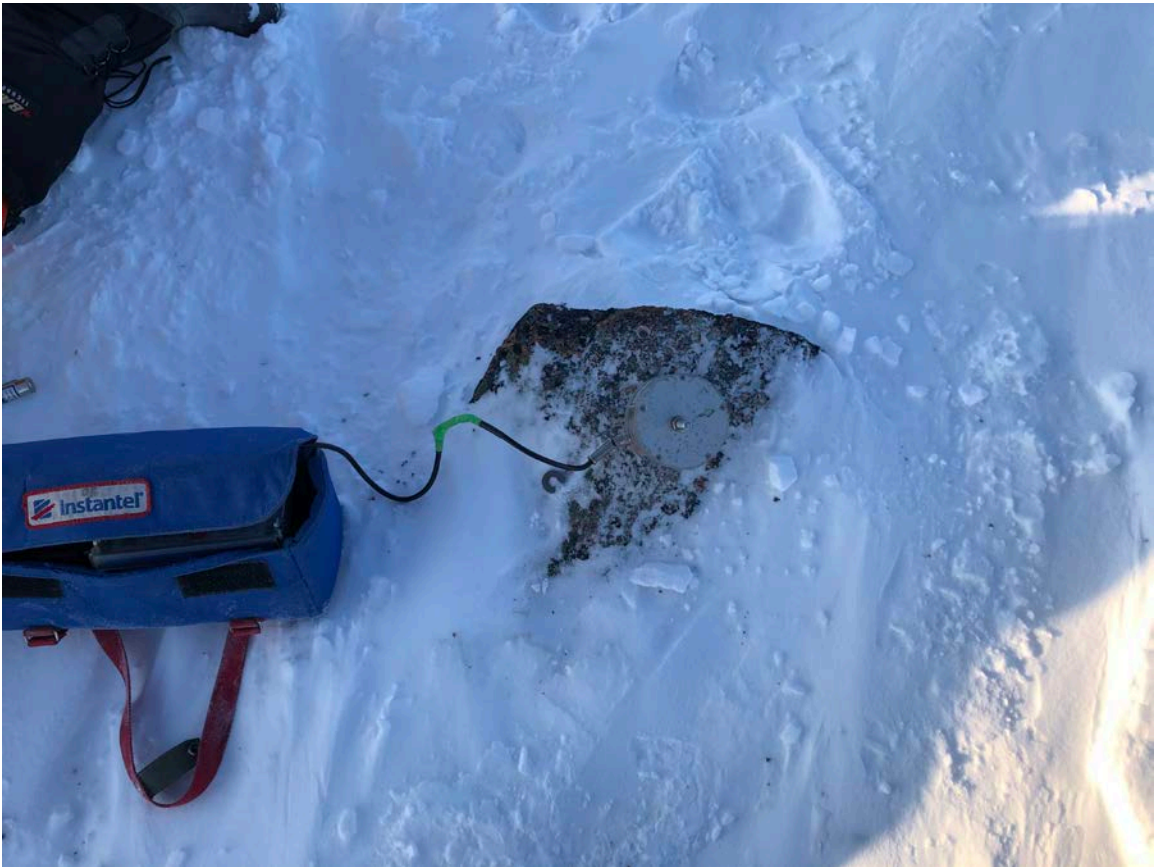
Figure 2 – Blast Monitoring Station installed with a rock anchor.
