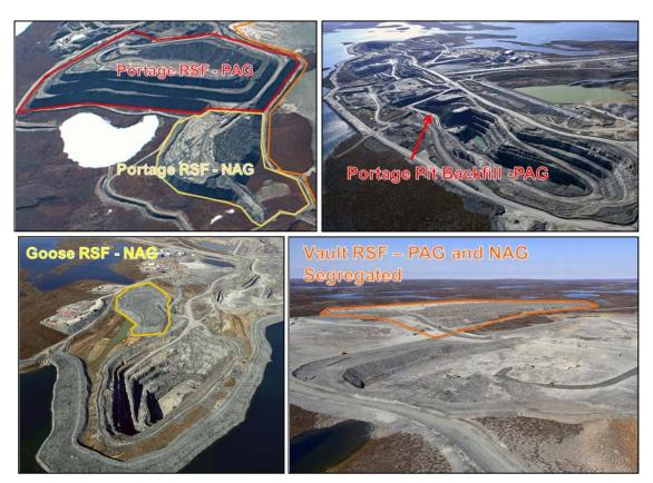
Figure 4: Waste Rock Storage Facilities at Meadowbank
