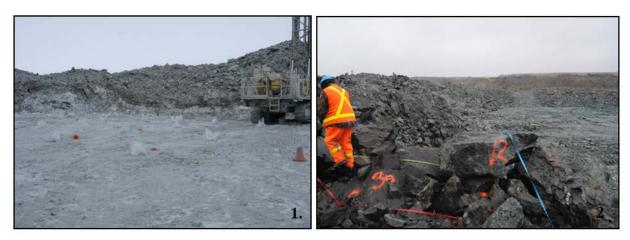
Photo 1: Preparation of the samples from drill cuttings Photo 2: Differentiation of PAG/NAG rock and ore after a blast based on laboratory results and blast pattern
