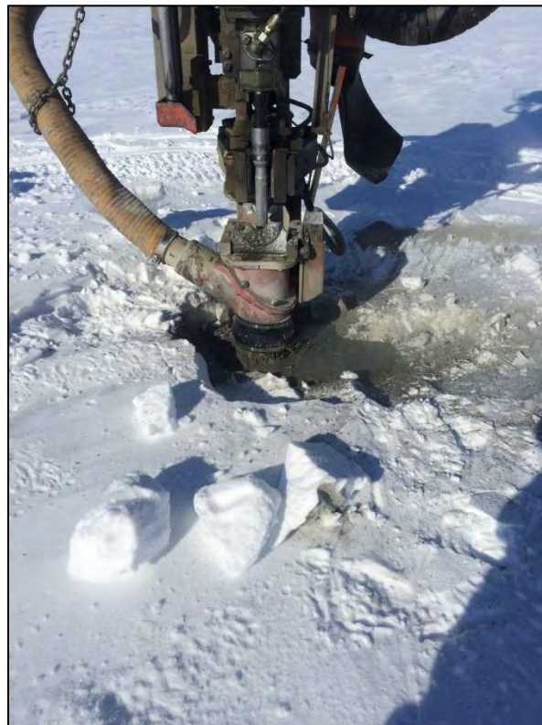
Figure 29: Presence of water in SWTC-19-10
