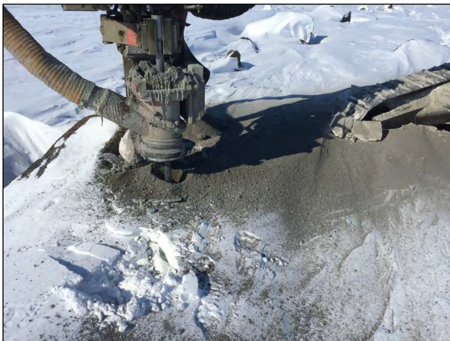
Figure 21: Poor bedrock drilling in SWTC-19-06
