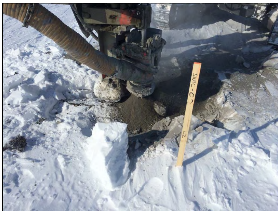
Figure 13: Overburden drilling in SWTC-19-02
