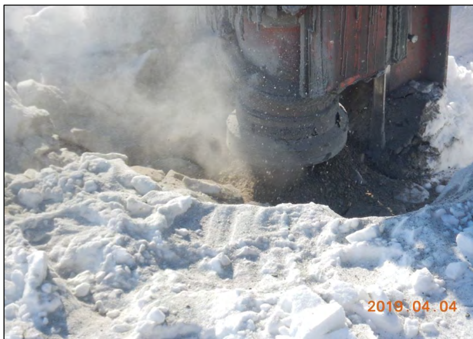
Figure 25: Overburden drilling in SWTC-19-08
