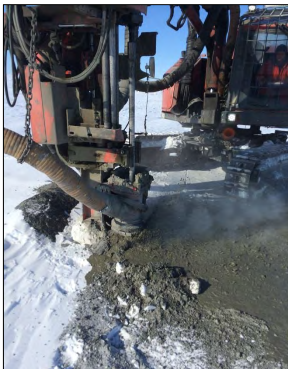
Figure 17: Presence of water in SWTC-19-04
