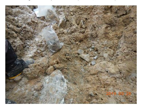
Figure 2: Soil sampling in a test pit (IVR-TP2, 2019-09-28).
