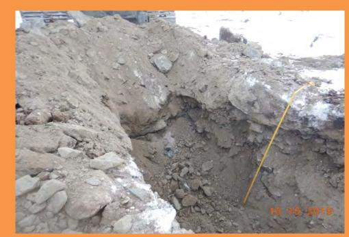
IVRWRSF-TP6 by B. Lessard Depth (m) Surveyed Coordinates (X,Y,Z): 608180.704,7256750.575,180.386 Organic topsoil Comments: 0.00 0.20 to Coarse gravel with pockets of fine sand, grey to brown, moist. Bedrock outcropping at 1.2 m on one side of the excavation. 0.20 to 1.70 3 samples: A (0.5 m), B (1.0 m), C (1.7 m) 1.70 to bedrock 1.70 Refusal (bedrock) Depth of Test Pit: Water: N/A
