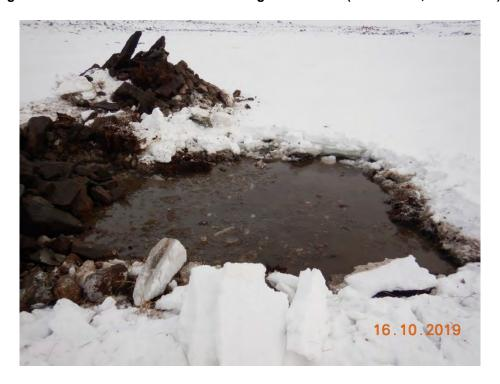
Figure 4: Flooded test pit (IVRWRSF-TP11, 2019-10-16).
