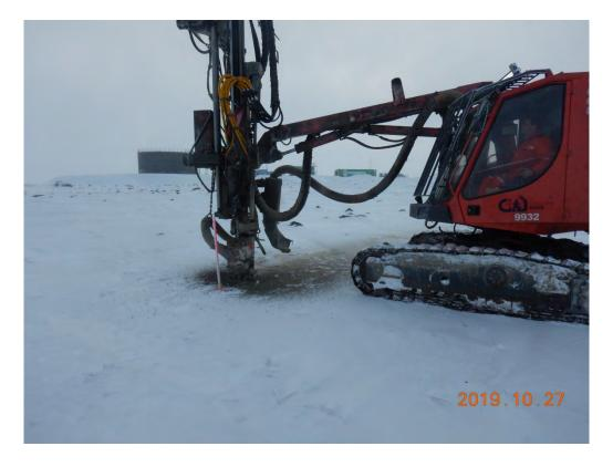
Figure 5: Bedrock sounding with a Tamrock drill (borehole #19, 2019-10-27).
