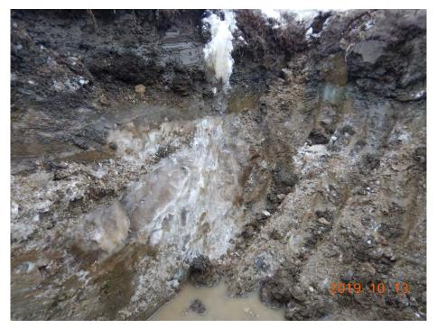
Figure 3: Presence of ice lenses indicating ice-rich soil (IVRDC-TP1, 2019-10-13).
