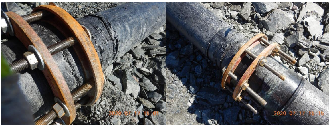
Photo 4. Flanged assembly without gasket
