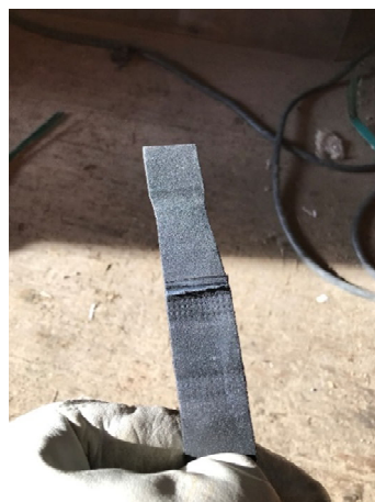
2082: (2021-03-16), Calibration peel test fracture result.
