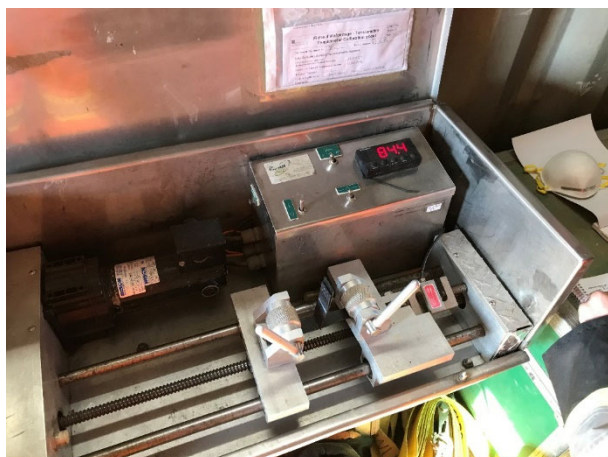
2081: (2021-03-16), Tensiometer peel test on calibration sample.
