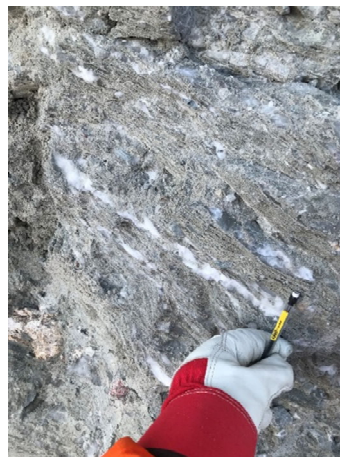
2064: (2021-03-12), looking S from Sta. 0+0+260. Close up view of ice lens in downstream trench wall.
