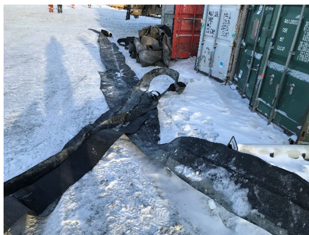
2211: (2021-04-17), Liner trimmings showing damaged hinge weld.
