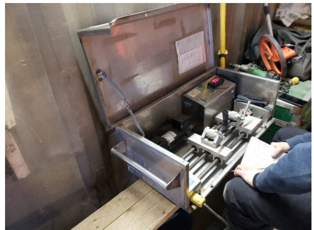
2112: (2021-03-24) Liner QC conducting first calibration test at 7 AM, loads at failure in peel and shear were greater than minimum values presented in Technical Specifications.
