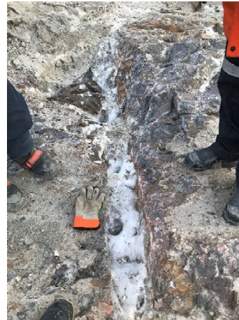
2192: (2021-04-10), looking N from Sta. 0+500. Ice-filled joint at Sta. 0+500 (joint #4 on bedrock map).
