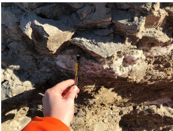
2061: (2021-03-12), looking N from Sta. 0+0+226. Ice seam in upstream trench.
