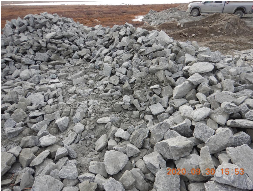
Photo 9. Non-compliant rip rap load, containing fines and gravel <100mm. Material on the photo has not been placed on the channel.
