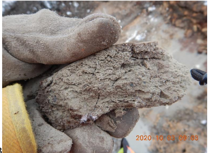
Photo 3. Foundation spot check STA 0+250, about 0.3m below grade. some ice visible at mm scale. Sample taken to confirm ice content.
