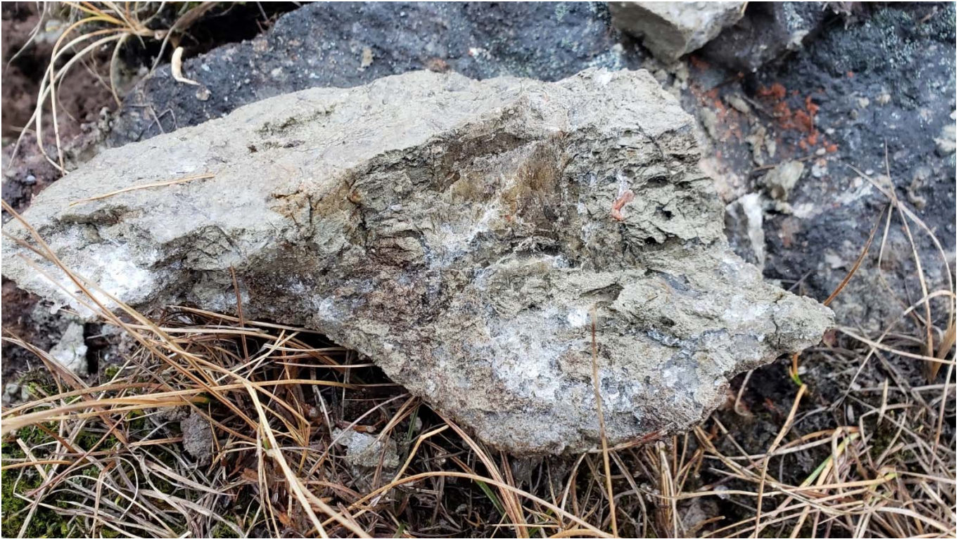
Photo 4: ice crystals and inclusion in till, from foundation at St. 0+243.
