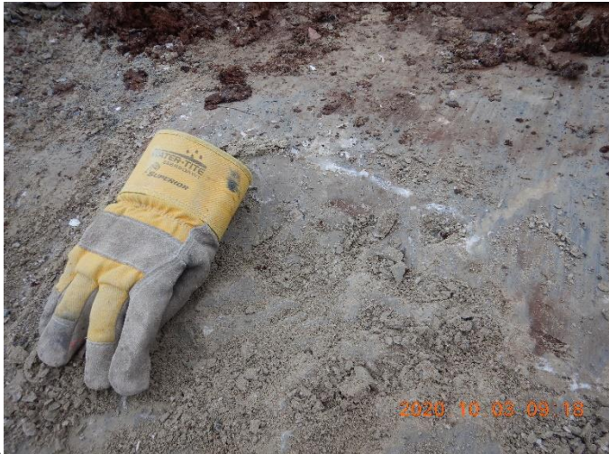
Photo 2. Foundation spot check STA 0+260, about 0.3m below grade. Visible presence of ice. Some ice lenses at mm scale and an isolated 1cm thick one.
