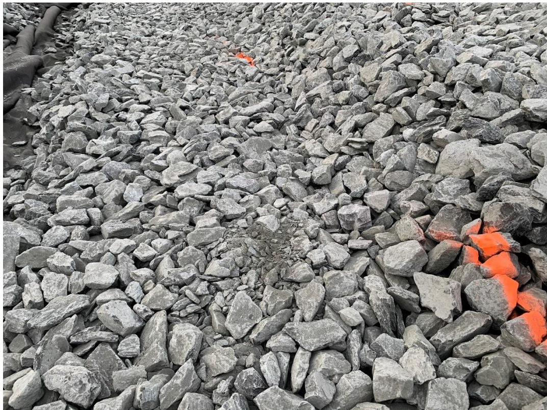
Figure 10: Riprap with too much fine material
