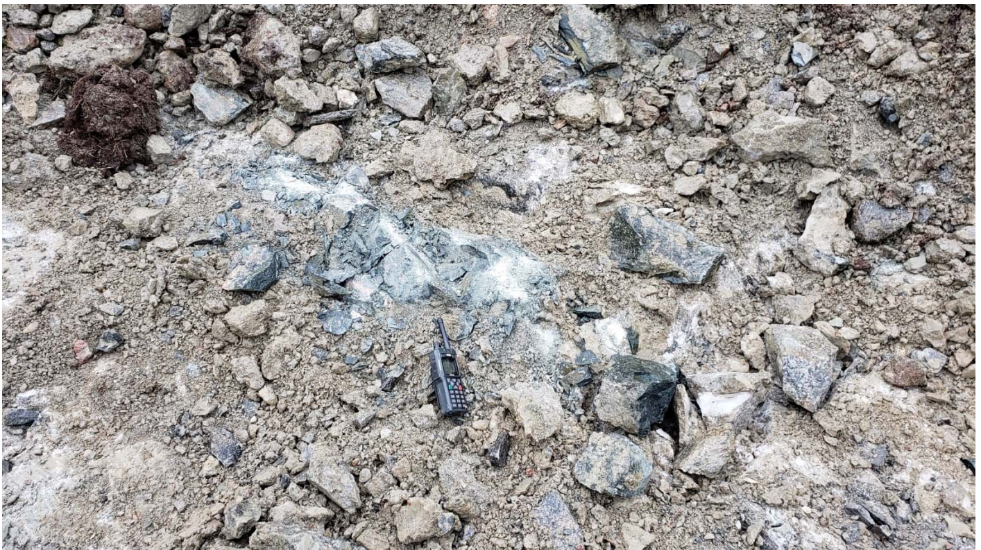
Photo 4: bedrock found at St.0+255. Estimate that about 10% of the surface was on bedrock.
