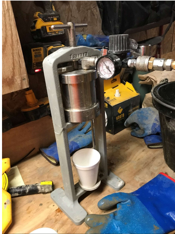
Performing Filtration test for Mix D
