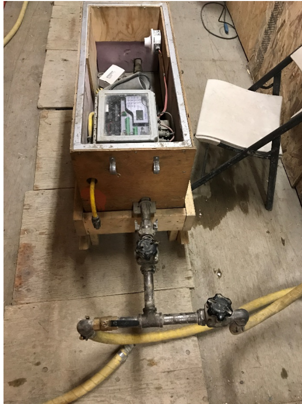
Acquisition system set up inside the injection unit
