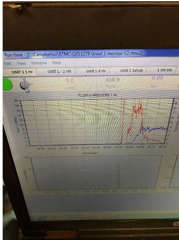
Screen shot of flow and pressure chart at S734.5 re-grout
