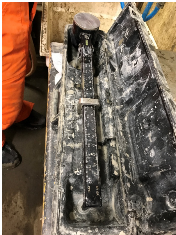
Taking specific gravity reading using mud balance
