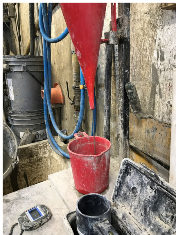
Measuring Marsh Value for Mix C.
