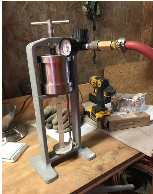
Photo 12: Performing Filtration Test
