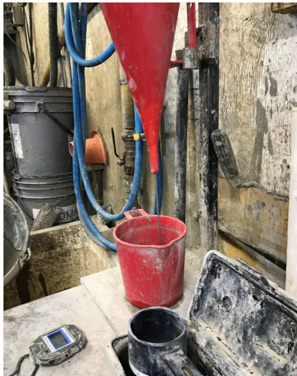
Photo 10: Performing marsh test to calculate marsh seconds
