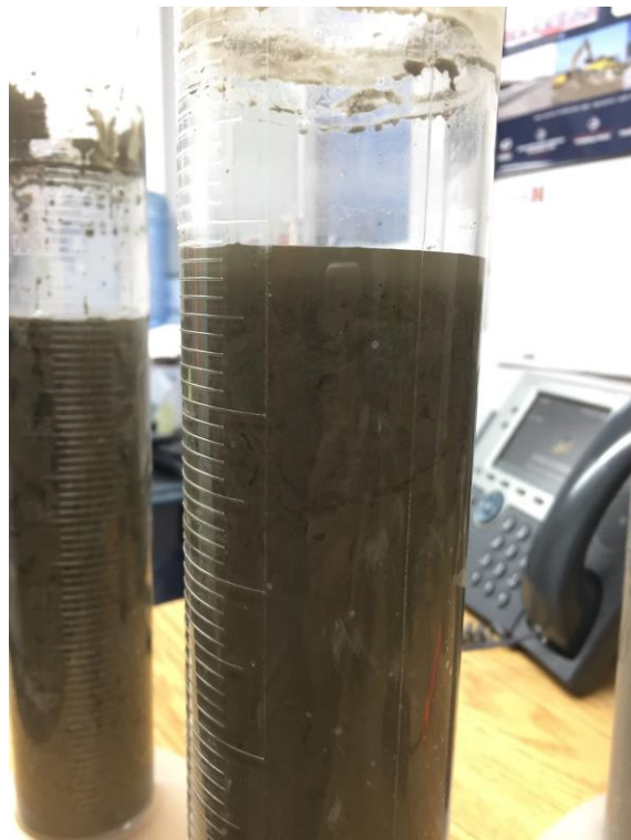
Figure 2: Mix A + cold weather admixture after ~ 2 hours
