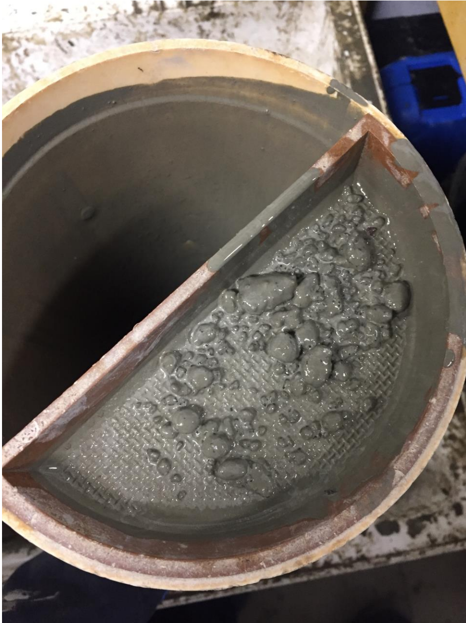
Figure 1: Chunks of Glenium 3030 NS observed on Marsh Funnel sieve (Mix A)
