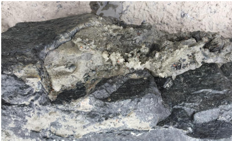
Indicators of Presence of Frozen Material above bedrock in the station between 0 + 555 and 0 + 595
