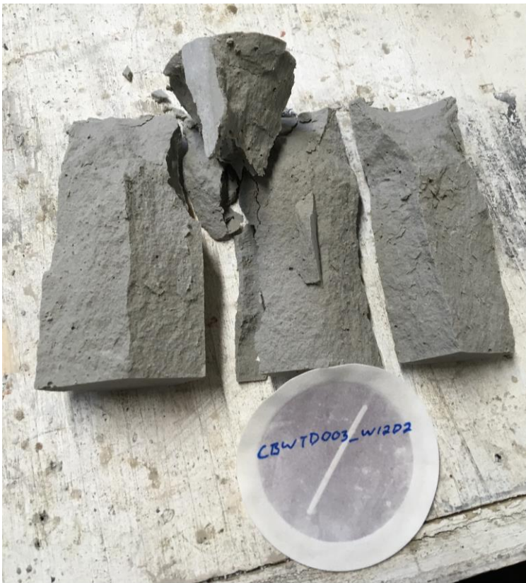
Figure 3: "Shear cone" observed on broken CB sample after unconfined compression test
