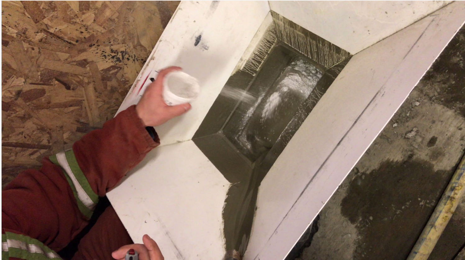
Adding Celbex manually into the open throat pump
