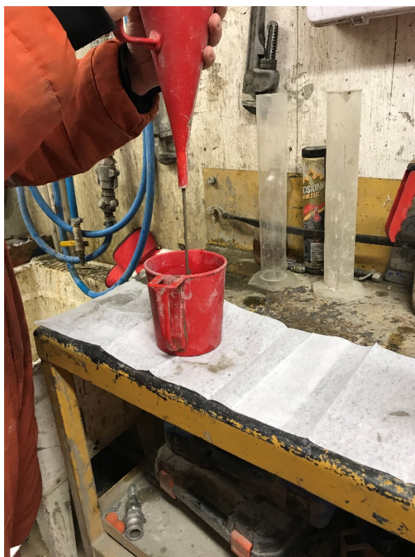
Checking marsh funnel time for grout
