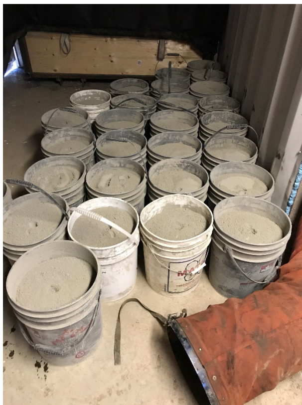
20 kg pails placed in the heated C-can
