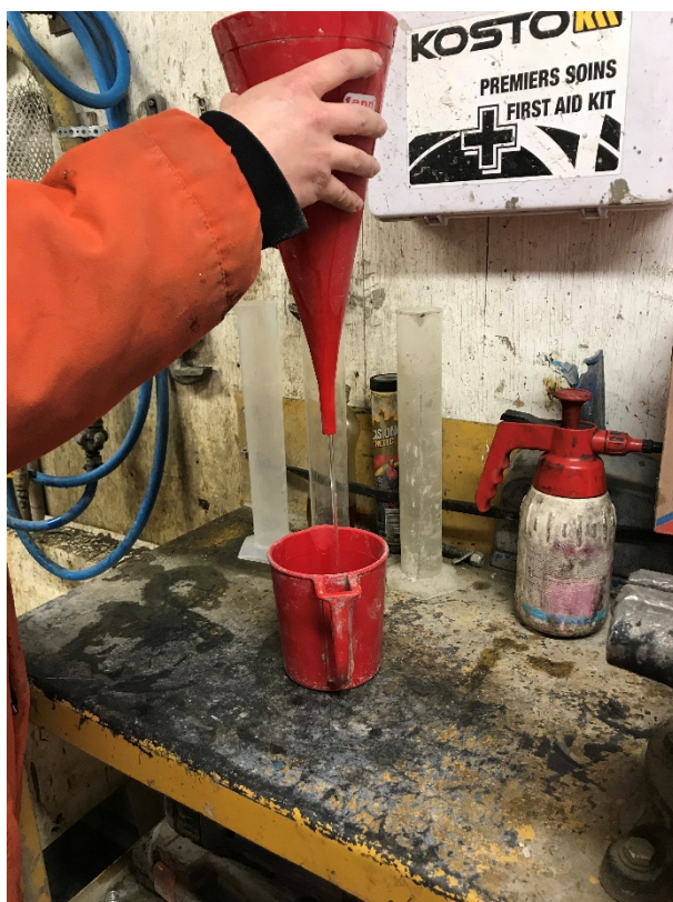
Calibrating Marsh funnel with water
