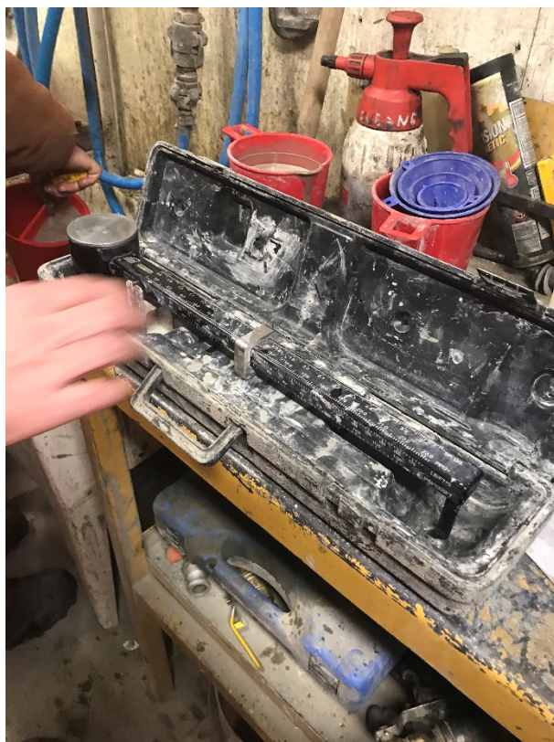
Checking Specific gravity of grout
